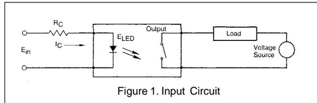
Figure 1. Input Circuit
