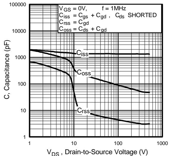
Fig. 1: Typical Capacitance Vs. Drain to Source Voltage
