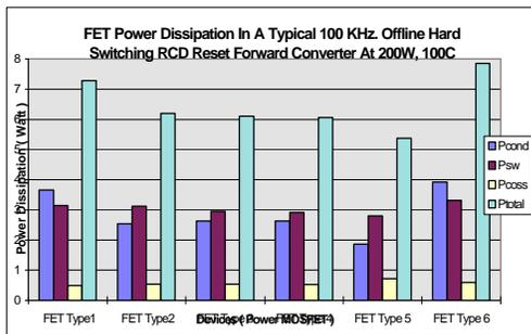
Fig. 4: FET Loss Distribution Comparison @ 100kHz.
