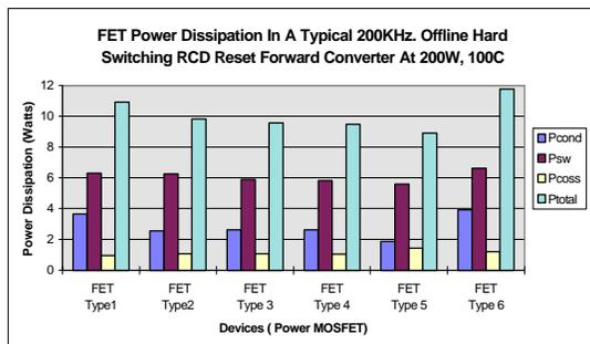
Fig. 5: FET Loss Distribution Comparison @ 200kHz.
