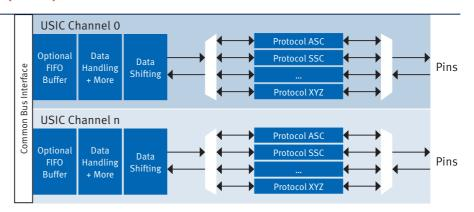
DESIGNERS CAN NOW CONFIGURE universal serial interfaces depending on their system's requirements. Whether UART, SSC (SPI compatible), LIN, IIC or IIS, any interface is possible after a quick adjustment of the USIC module.
