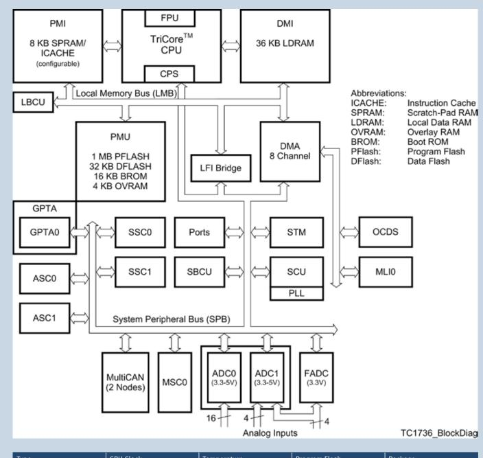
TypeCPU ClockTemperatureProgram FlashPackageSAK-TC1736-128F80HL80MHz-40/125°C1MBQFP-144
