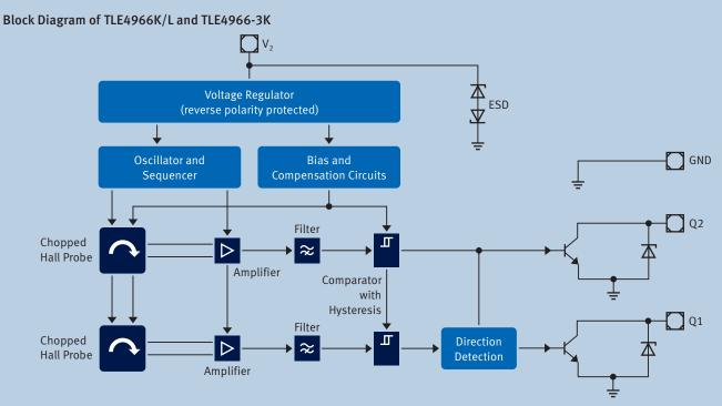
Block Diagram of TLE4966K/L and TLE4966-3K double Hall Sensor with direction detection. The distance of the Hall elements on the chip is 1.45mm.
