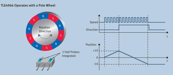
The number of pole pairs defines the positioning accuracy of the system.
