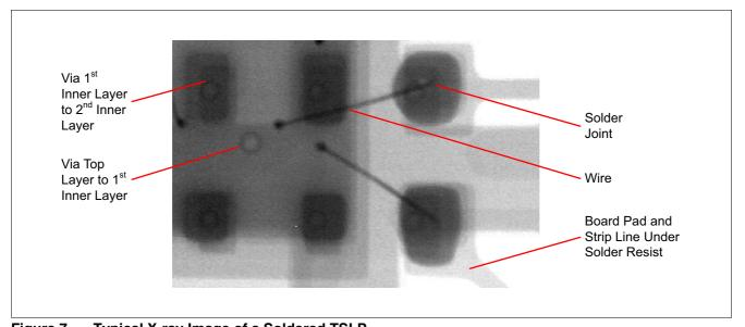
Figure 7 Typical X-ray Image of a Soldered TSLP.
