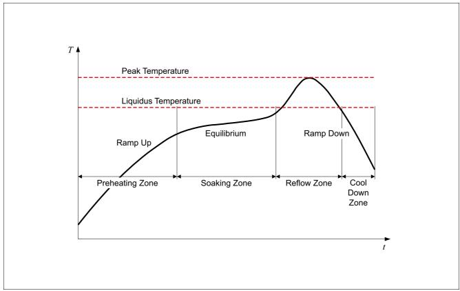
Figure 5 General Forced Convection Reflow Solder Profile
