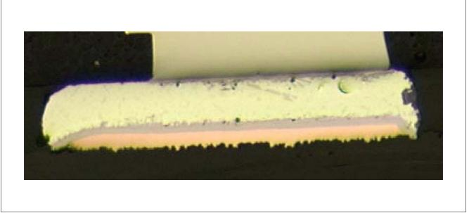
Figure 8 Cross Section of a TSLP Solder Joint (Pb-free)
