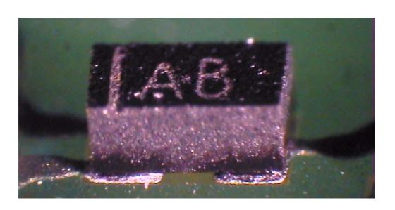
Figure 6 Typical Side View of TSLP Solder Joints
