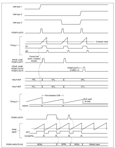
Figure 24-7 Hall Sensor timing diagram
