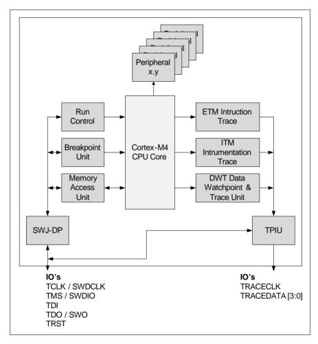
Figure 27-1 Debug and Trace System block diagram
