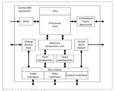
Figure 2-1 Cortex-M4 Block Diagram
