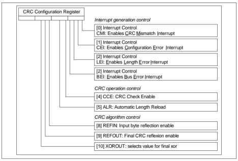
Figure 6-2 CRC kernel configuration register
