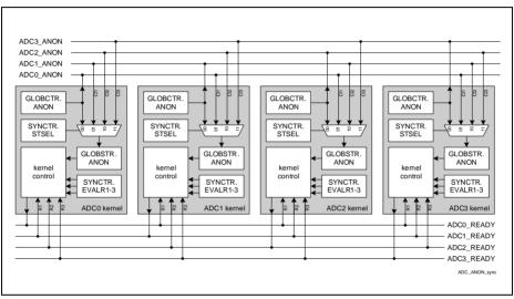
Figure 19-24 Synchronization via ANON and Ready Signals
