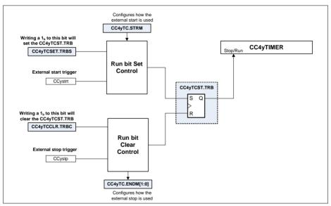
Figure 22-5 Timer start/stop control diagram
