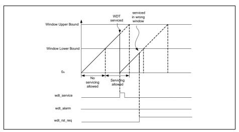
Figure 9-4 Reset upon servicing in a wrong window
