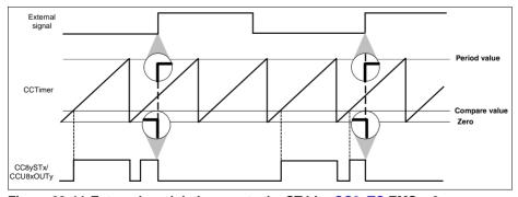
Figure 23-44 External modulation resets the ST bit - CC8yTC.EMS =  $0_B$
