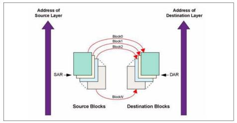
Figure 5-20 Multi-Block DMA Transfer with Source and Destination Address
