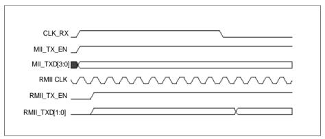
Figure 15-23 Start of MII and RMII Transmission in 10 Mbit/s Mode
