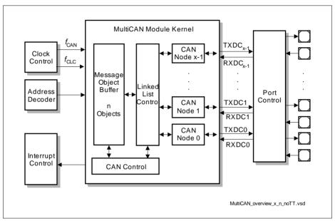
Figure 18-1 **Overview of the MultiCAN Module**
