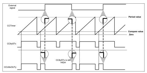
Figure 23-46 External modulation gating the output - CC8yTC.EMT = 1<sub>B</sub>
