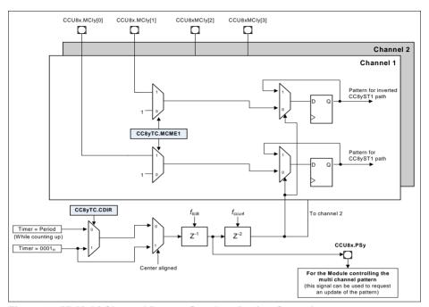
Figure 23-55 Multi Channel Pattern Synchronization Control
