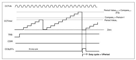
Figure 23-75 PWM with 0% duty cycle - Edge Aligned Mode
