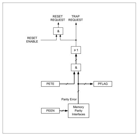
Figure 11-3 Parity Error Control Logic
