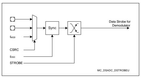
Figure 20-5 Demodulator Data Strobe Selection
