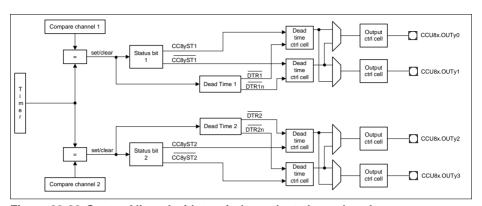
Figure 23-26 Center Aligned with two independent channels scheme
