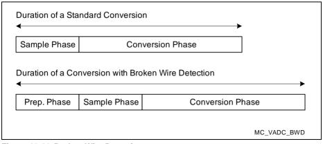
Figure 19-26 Broken Wire Detection
