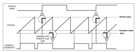
Figure 23-45 External modulation clearing the ST bit - CC8yTC.EMS = 1<sub>B</sub>
