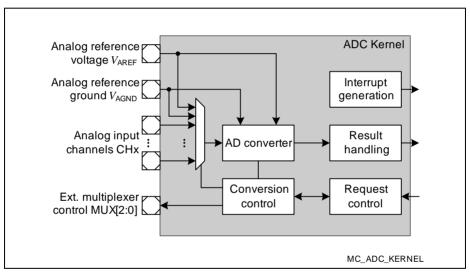
Figure 19-2 ADC Kernel Block Diagram
