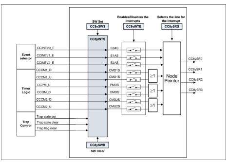
Figure 23-87 Slice interrupt node pointer overview
