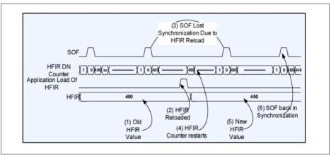
Figure 16-7 Functionality when HFIRRIdCtrl = 0<sub>B</sub>
