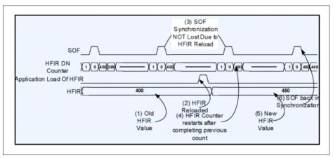
Figure 16-8 Functionality when HFIRRIdCtrl = 1<sub>B</sub>
