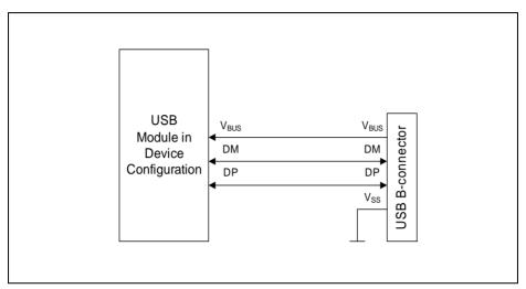
Figure 16-4 USB Device Connections
