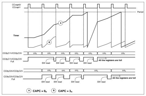
Figure 23-80 Capture mode usage - single channel
