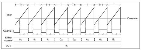
Figure 23-67 Dither timing diagram in edge aligned - CC8yTC.DITHE = 11<sub>B</sub>
