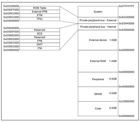
Figure 7-1 Cortex-M4 processor address space
