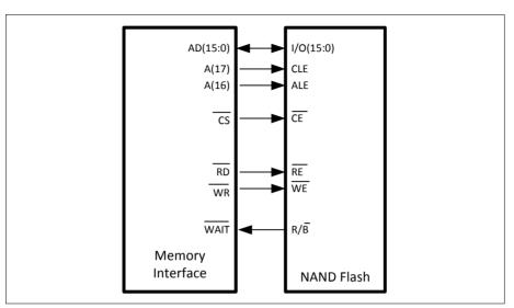
Figure 14-20 Example of interfacing a Nand Flash device to the Memory Controller
