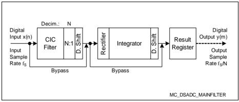
Figure 20-7 Structure of the Main Filter Chain
