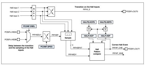
Figure 24-3 Hall Sensor Control Diagram
