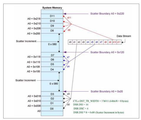
Figure 5-6 Example of Destination Scatter Transfer
