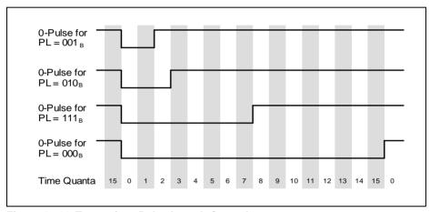
Figure 17-33 Transmitter Pulse Length Control
