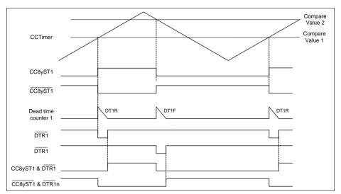
Figure 23-29 Asymmetric Center aligned mode with dead time
