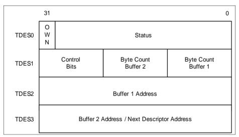
Figure 15-8 Transmit Descriptor Format
