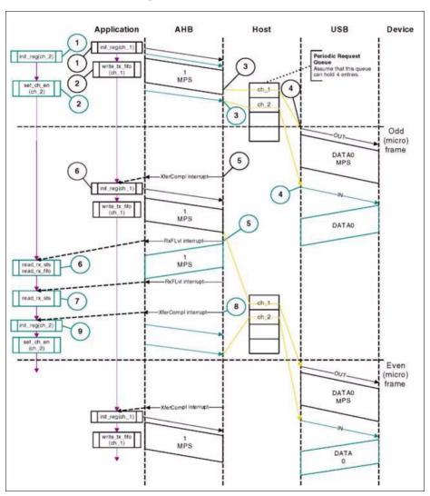
Figure 16-13 Normal Isochronous OUT/IN Transactions in Slave Mode
