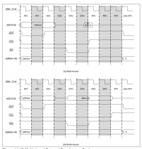
Figure 14-17 Multiplexed External Bus Access Cycles
