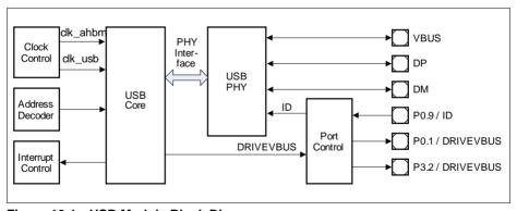
Figure 16-1 USB Module Block Diagram
