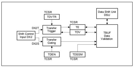
Figure 17-18 Transmit Data Validation
