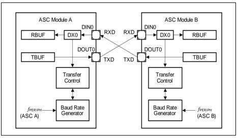
Figure 17-29 ASC Signal Connections for Full-Duplex Communication
