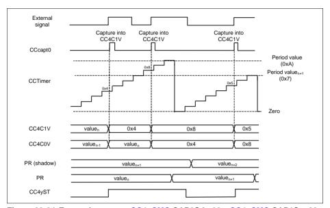
Figure 22-24 External capture - CC4yCMC.CAP0S != 00<sub>B</sub>, CC4yCMC.CAP1S = 00<sub>B</sub>
