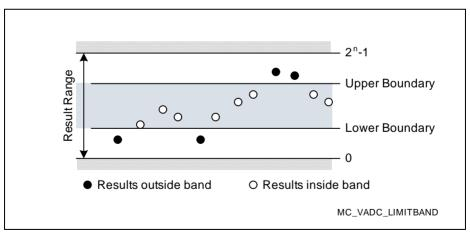
Figure 19-11 Result Monitoring through Limit Checking
