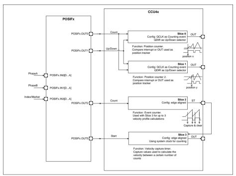
Figure 24-18 Quadrature Decoder Mode usage - profile 2
