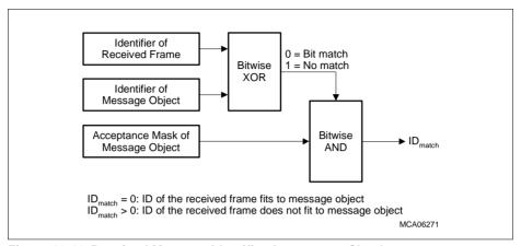
Figure 18-13 Received Message Identifier Acceptance Check
