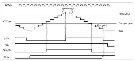
Figure 23-15 Single shot center aligned - CC8yTC.TSSM = 1<sub>B</sub>, CC8yTC.TCM = 1<sub>B</sub>
