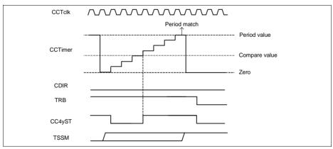
Figure 22-14 Single shot edge aligned - CC4yTC.TSSM = 1<sub>B</sub>, CC4yTC.TCM = 0<sub>B</sub>
