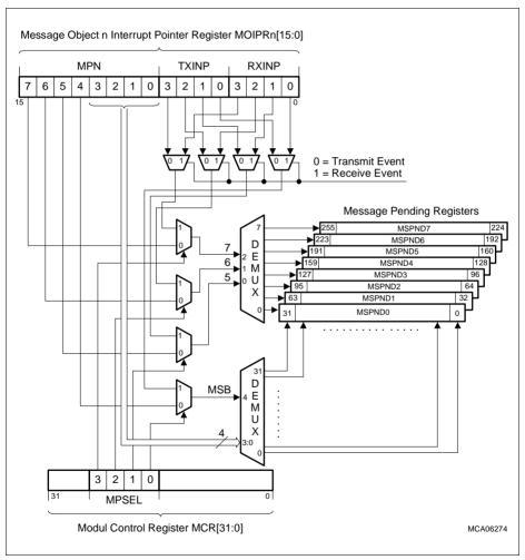
Figure 18-16 Message Pending Bit Allocation
