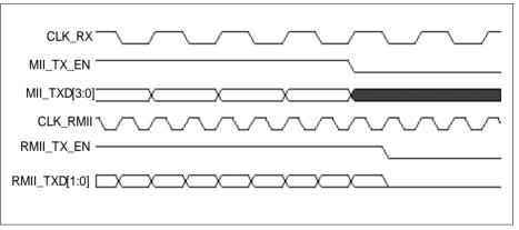
Figure 15-22 End of MII and RMII Transmission in 100 Mbit/s Mode
