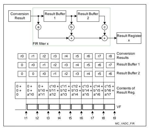
Figure 19-20 FIR Filter Structure
