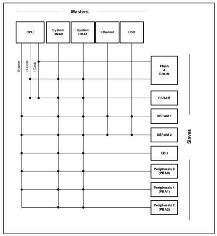
Figure 3-1 Multilayer Bus Matrix
