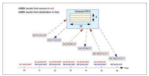
Figure 5-8 Breakdown of Block Transfer
