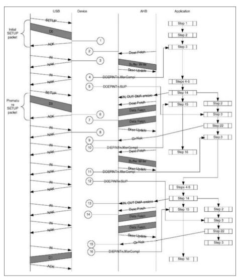
Figure 16-48 Premature SETUP During Control Read Data Phase
