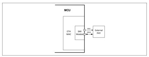
Figure 15-14 SMA Interface Block
