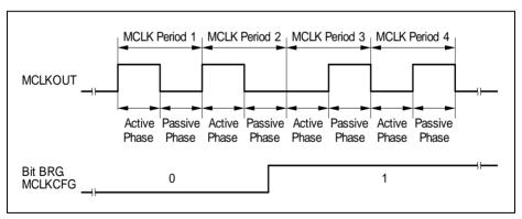
Figure 17-16 Master Clock Output Configuration
