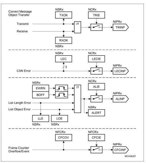
Figure 18-9 CAN Node Interrupts
