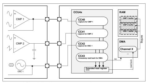
Figure 22-64 Extended read usage scheme example
