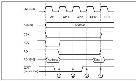
Figure 14-18 External Wait Insertion (Synchronous Mode)
