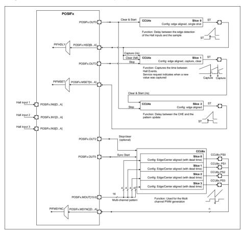
Figure 24-16 Hall Sensor Mode usage - profile 2
