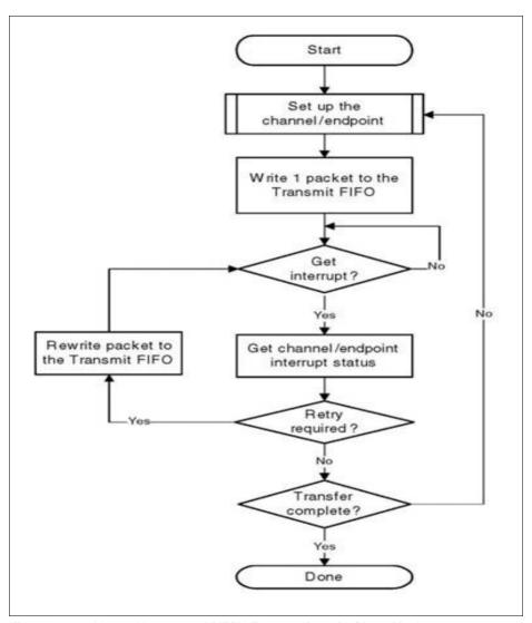
Figure 16-12 Normal Interrupt OUT/IN Transactions in Slave Mode Interrupt Service Routine for Interrupt OUT Transactions in Slave Mode
