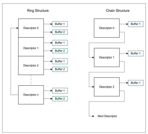
Figure 15-2 Descriptor Ring and Chain Structure
