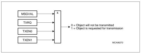
Figure 18-14 Effective Transmit Request of Message Object
