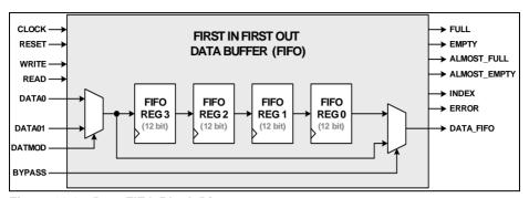
Figure 21-3 Data FIFO Block Diagram
