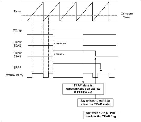
Figure 23-48 Trap timing diagram, CC8yTCST.CDIR = 0 CC8yPSL.PSL = 0
