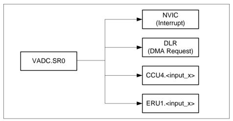
Figure 4-2 Example for Service Request Distribution
