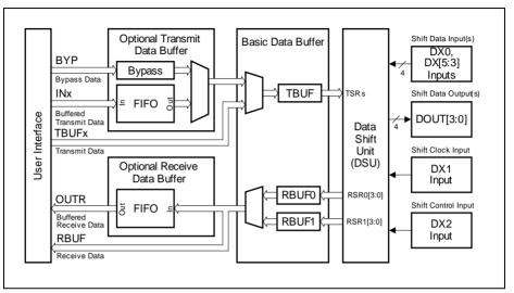
Figure 17-3 Principle of Data Buffering
