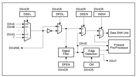
Figure 17-11 Input Conditioning for DX[2:1]
