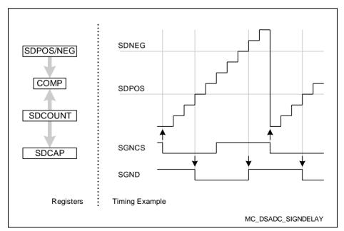
Figure 20-13 Sign Delay Example
