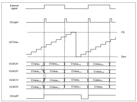
Figure 22-27 External Capture - CC4yTC.SCE = 1<sub>B</sub>
