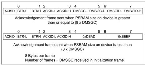
Figure 26-14 CAN Acknowledgement Frame
