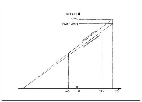
Figure 11-6 Gain adjustment of the RESULT curve
