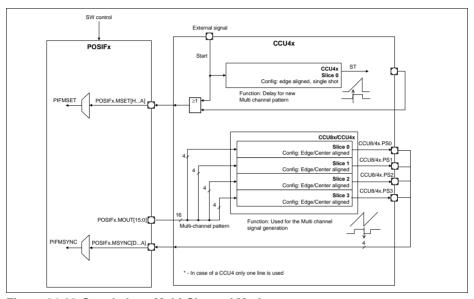
Figure 24-22 Stand-alone Multi-Channel Mode usage
