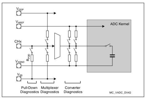
Figure 19-27 Signal Path Test
