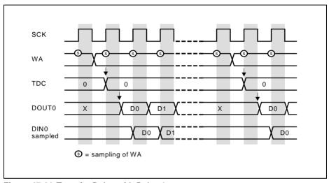
Figure 17-61 Transfer Delay with Delay 1
