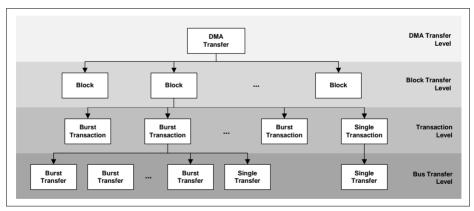
Figure 5-2 Transfer Hierarchy for Peripherals
