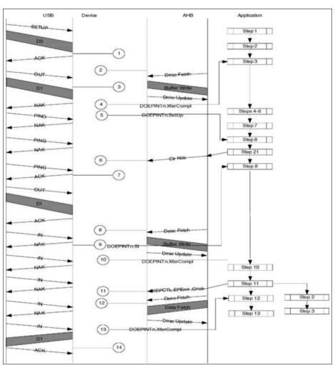
Figure 16-49 Premature Status Phase During Control Write
