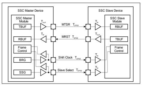
Figure 17-47 SSC Master Mode with Delay Compensation
