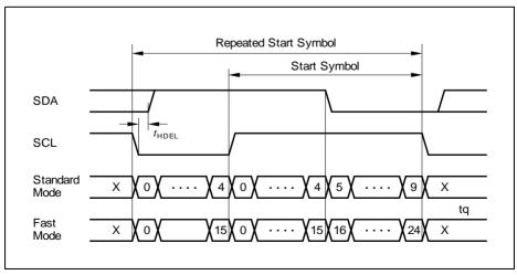
Figure 17-52 Repeated Start Symbol Timing
