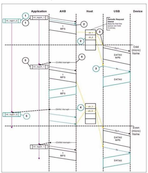
Figure 16-17 Normal Isochronous OUT/IN Transactions in DMA Mode
