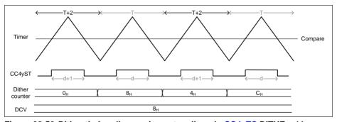
Figure 22-52 Dither timing diagram in center aligned - CC4yTC.DITHE = 11<sub>B</sub>
