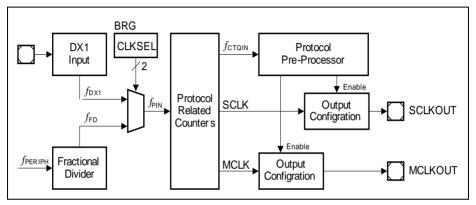
Figure 17-2 Baud Rate Generator
