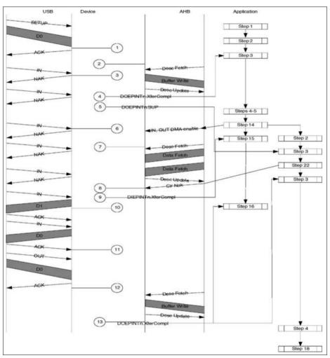
Figure 16-41 Three-Stage Control Read
