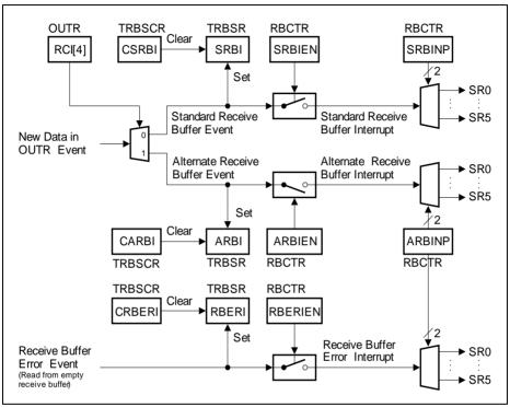
Figure 17-26 Receiver Buffer Events in RCI Mode
