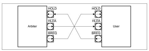
Figure 14-11 Connection of Bus Arbitration Signals
