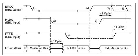
Figure 14-14 Arbitration Sequence with the EBU in Participant Mode
