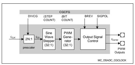
Figure 20-11 Carrier Generator Block Diagram
