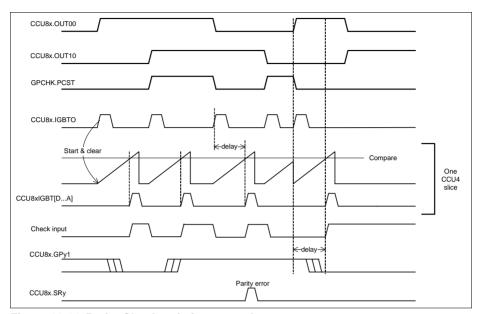
Figure 23-86 Parity Checker timing example
