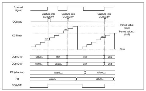
Figure 23-39 External capture - CC8yCMC.CAP0S != 00<sub>B</sub>, CC8yCMC.CAP1S = 00<sub>B</sub>
