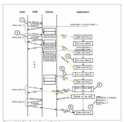
Figure 16-22 Two-Stage Control Transfer
