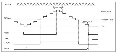
Figure 22-15 Single shot center aligned - CC4yTC.TSSM = 1<sub>B</sub>, CC4yTC.TCM = 1<sub>B</sub>
