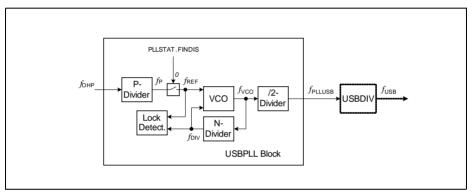
Figure 11-24 PLLUSB Block Diagram
