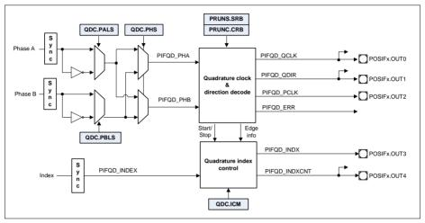
Figure 24-9 Quadrature Decoder Control Overview
