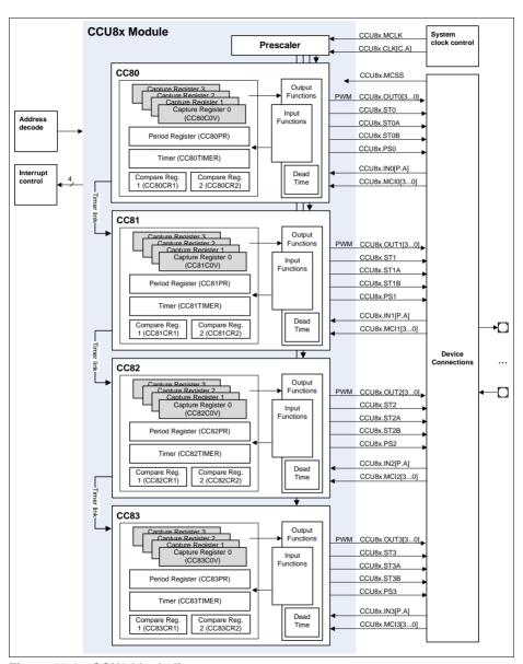
Figure 23-1 CCU8 block diagram
