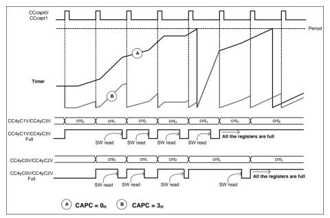
Figure 22-62 Capture mode usage - single channel
