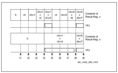
Figure 19-19 Standard Data Reduction Filter with FIFO Enabled
