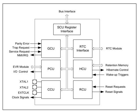
Figure 11-1 SCU Block Diagram
