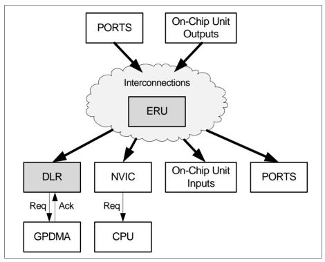
Figure 4-1 Block Diagram on Service Request Processing
