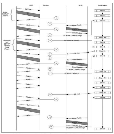
Figure 16-47 Premature SETUP During Control Write Data Phase
