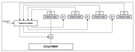
Figure 22-28 Slice Capture Logic - CC4yTC.SCE =  $1_B$
