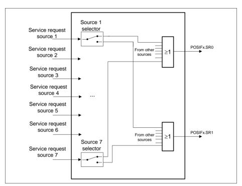
Figure 24-26 Interrupt node pointer overview - quadrature decoder mode
