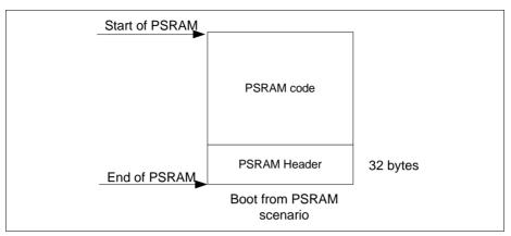
Figure 26-8 PSRAM Layout for PSRAM Boot
