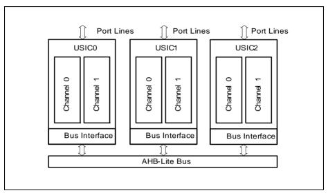
Figure 17-65 USIC Module Structure in XMC4500
