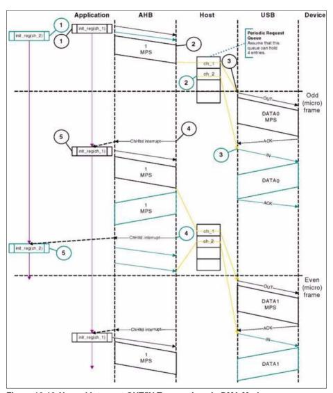
Figure 16-16 Normal Interrupt OUT/IN Transactions in DMA Mode
