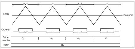
Figure 22-50 Dither timing diagram in center aligned - CC4yTC.DITHE = 01<sub>B</sub>
