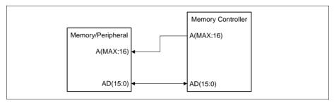
Figure 14-6 Connection of a 16-bit Multiplexed Device to Memory Controller
