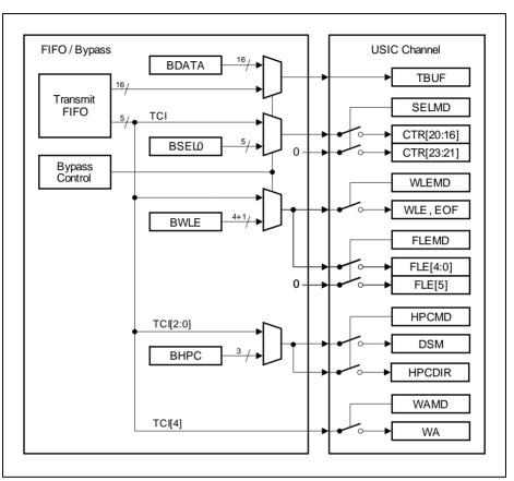
Figure 17-28 TCI Handling with FIFO / Bypass
