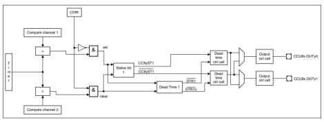
Figure 23-28 Center Aligned Asymmetric mode scheme
