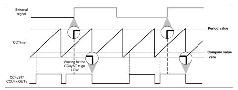
Figure 22-30 External modulation clearing the ST bit - CC4yTC.EMT =  $0_B$ , CC4yTC.EMS =  $1_B$
