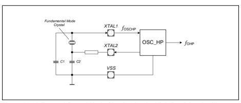
Figure 11-21 External Crystal Mode Circuitry for the High-Precision Oscillator
