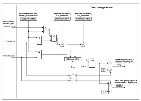
Figure 23-18 Dead Time generator scheme
