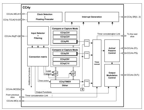
Figure 22-2 CCU4 slice block diagram
