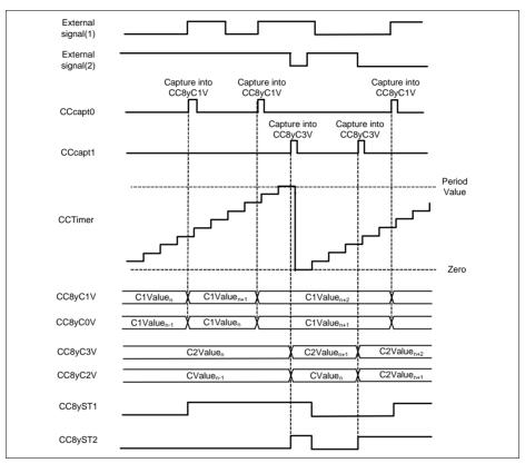
Figure 23-40 External capture - CC8yCMC.CAP0S != 00<sub>B</sub>, CC8yCMC.CAP1S != 00<sub>B</sub>
