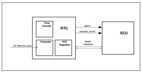
Figure 10-1 Real-Time Clock Block Diagram Structure
