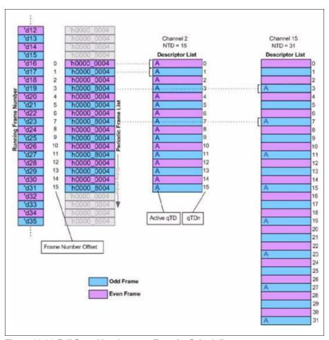
Figure 16-21 Full Speed Isochronous Transfer Scheduling
