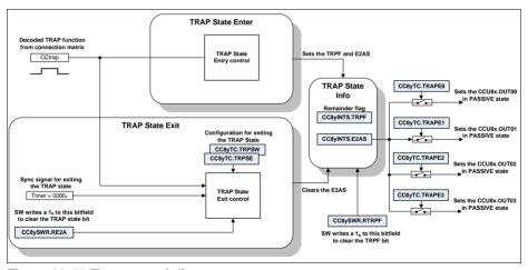
Figure 23-47 Trap control diagram
