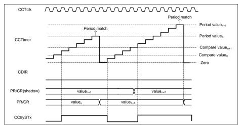
Figure 23-12 Edge aligned mode,  $CC8yTC.TCM = 0_B$
