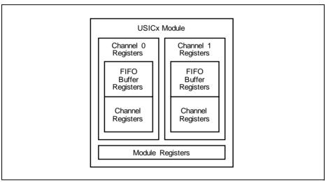
Figure 17-64 USIC Module and Channel Registers
