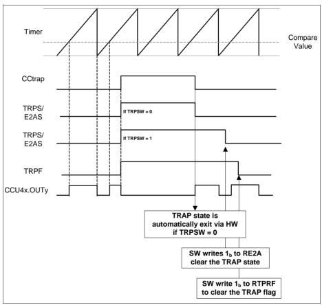
Figure 22-33 Trap timing diagram, CC4yPSL.PSL = 0<sub>B</sub> (output passive level is 0<sub>B</sub>)
