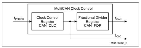
Figure 18-23 MultiCAN Module Clock Generation
