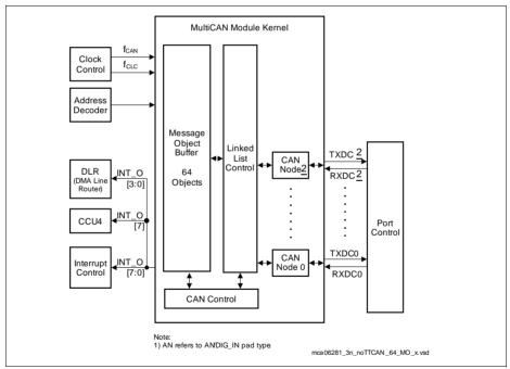
Figure 18-27 CAN module Implementation and Interconnections
