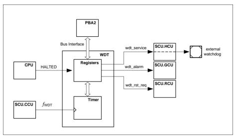
Figure 9-1 Watchdog Timer Block Diagram
