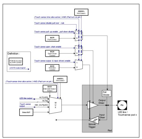
Figure 12-8 Over-rule Control on Pin for Touch-Sense Function
