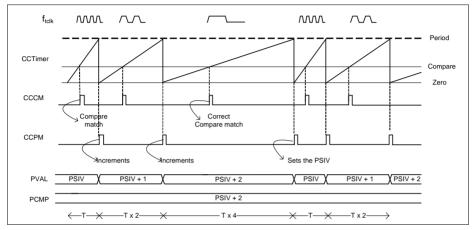
Figure 22-60 Floating Prescaler compare mode usage - Edge Aligned
