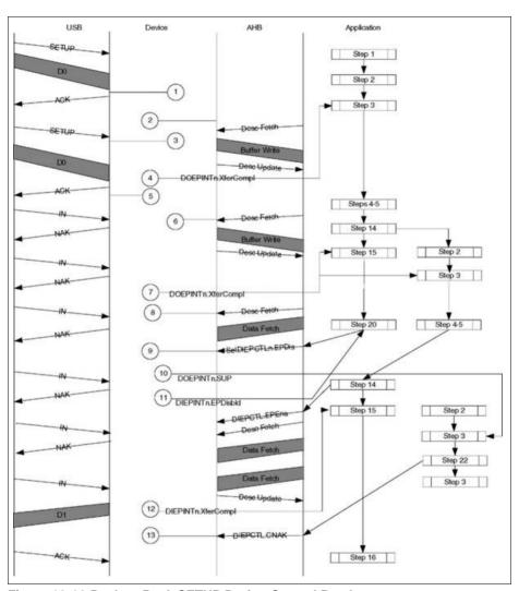
Figure 16-44 Back-to-Back SETUP During Control Read
