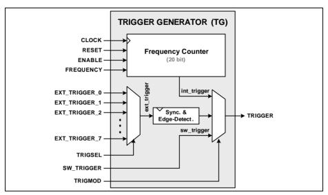
Figure 21-2 Trigger Generator Block Diagram
