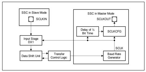
Figure 17-38 SSC Shift Clock Signals
