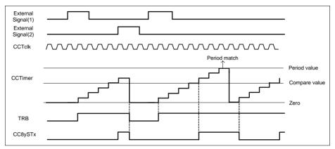
Figure 23-33 Start (as start)/ stop (as flush and stop) -  $CC8yTC.STRM = 0_B$ ,  $CC8yTC.ENDM = 10_B$
