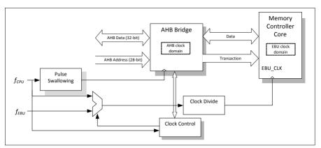
Figure 14-5 AHB/Memory Controller Clocking Domains (Simplified Block Diagram)
