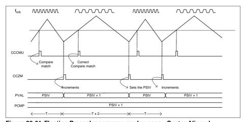
Figure 22-61 Floating Prescaler compare mode usage - Center Aligned
