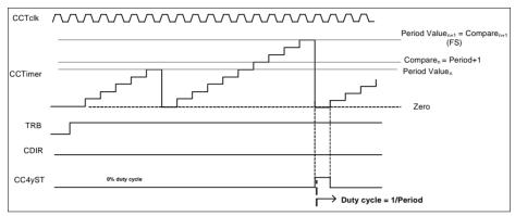
Figure 22-57 PWM with 0% duty cycle - Edge Aligned Mode
