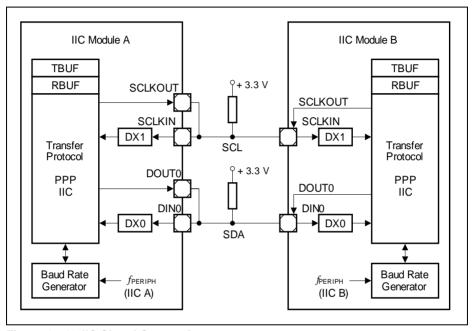
Figure 17-49 IIC Signal Connections
