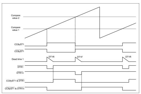
Figure 23-24 Edge Aligned - Asymmetric PWM timing, CC8yCR1.CR1 < CC8yCR2.CR2
