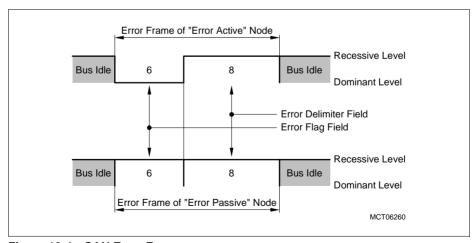
Figure 18-4 CAN Error Frames
