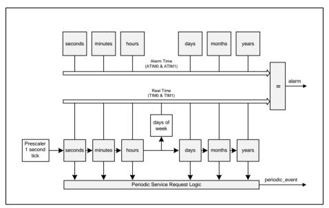
Figure 10-2 Block Diagram of RTC Time Counter
