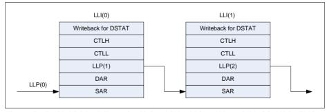
Figure 5-15 Multi-Block Transfer Using Linked Lists When CFG.SS\_UPD\_EN is set to '0'
