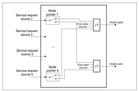
Figure 24-24 Interrupt node pointer overview - hall sensor mode
