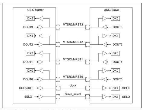
Figure 17-43 Connections for Quad-SSC Example
