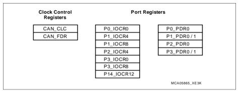
Figure 18-25 CAN Implementation-specific Special Function Registers
