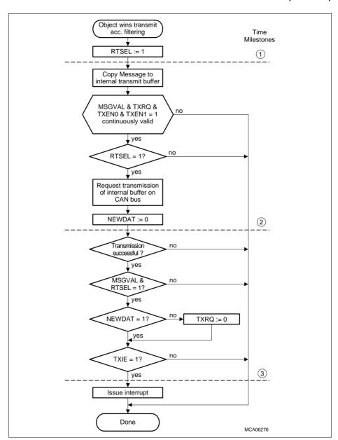
Figure 18-18 Transmission of a Message Object
