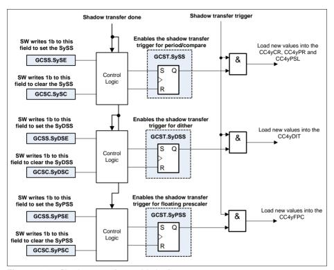
Figure 22-9 Shadow transfer enable logic
