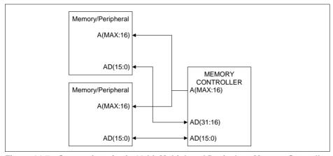
Figure 14-7 Connection of twin 16-bit Multiplexed Device's to Memory Controller
