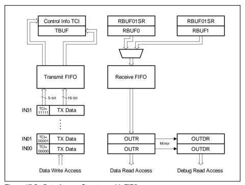
Figure 17-5 Data Access Structure with FIFO
