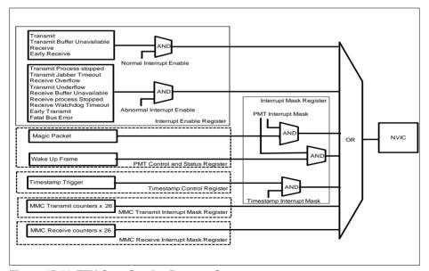
Figure 15-29 ETH Core Service Request Structure
