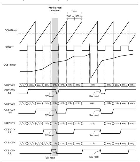
Figure 23-81 Three Capture profiles - CC8yTC.SCE = 1<sub>B</sub>
