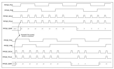
Figure 24-12 Quadrature clock and direction timings
