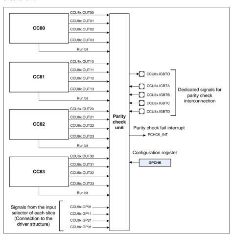
Figure 23-61 Parity checker structure
