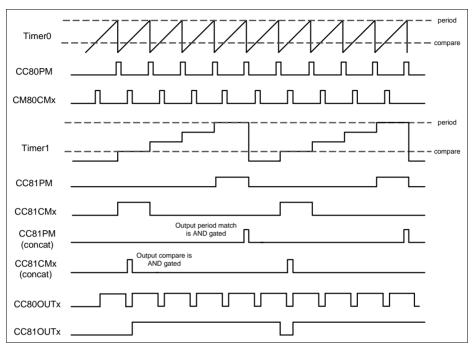
Figure 23-59 32 bit concatenation timing diagram
