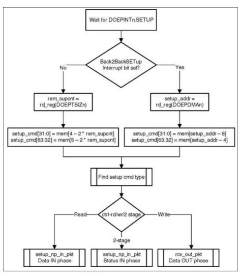
Figure 16-24 Processing a SETUP Packet
