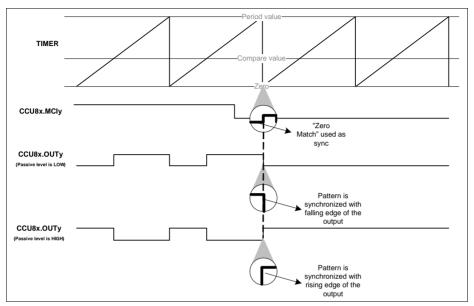
Figure 23-51 Multi channel pattern synchronization
