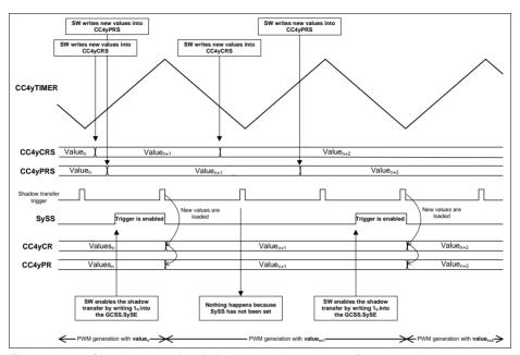
Figure 22-10 Shadow transfer timing example - center aligned mode
