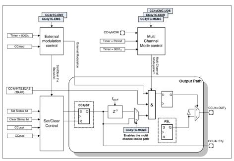
Figure 22-38 CC4y Status bit and Output Path
