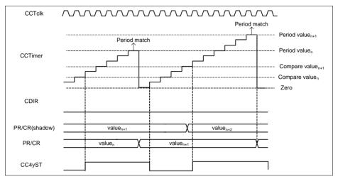
Figure 22-12 Edge aligned mode,  $CC4yTC.TCM = 0_B$
