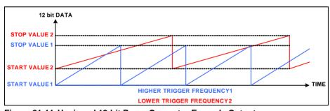
Figure 21-11 Unsigned 12-bit Ramp Generator Example Output
