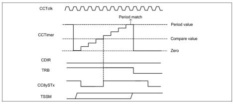
Figure 23-14 Single shot edge aligned -  $CC8yTC.TSSM = 1_B$ ,  $CC8yTC.TCM = 0_B$
