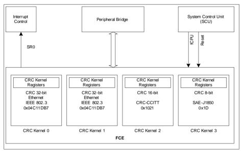
Figure 6-1 FCE Block Diagram
