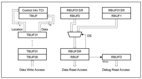
Figure 17-4 Data Access Structure without additional Data Buffer
