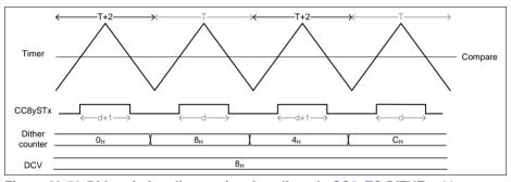
Figure 23-70 Dither timing diagram in edge aligned - CC8yTC.DITHE = 11<sub>B</sub>
