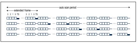
Figure 12-6 Hardware-Controlled Pad Turns for Autoscan of Four TSIN[x] with Extended Frames
