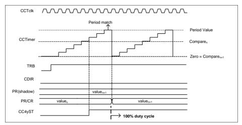
Figure 22-55 PWM with 100% duty cycle - Edge Aligned Mode
