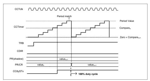
Figure 23-73 PWM with 100% duty cycle - Edge Aligned Mode
