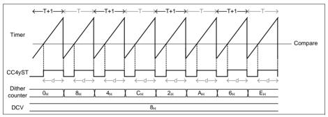
Figure 22-49 Dither timing diagram in edge aligned - CC4yTC.DITHE = 11<sub>B</sub>
