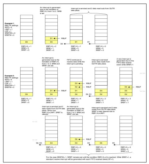
Figure 17-24 Standard Receive Buffer Event Examples
