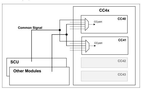
Figure 22-6 Starting multiple timers synchronously
