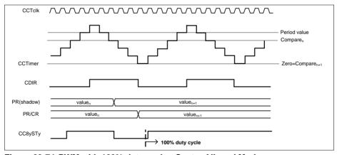
Figure 23-74 PWM with 100% duty cycle - Center Aligned Mode
