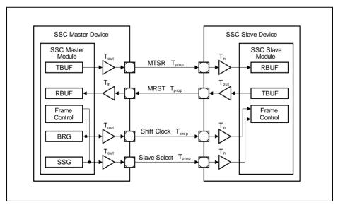
Figure 17-45 SSC Closed-loop Delay
