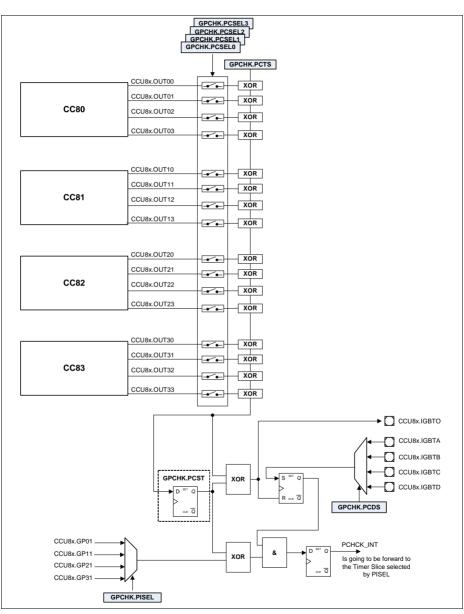
Figure 23-62 Parity checker logic
