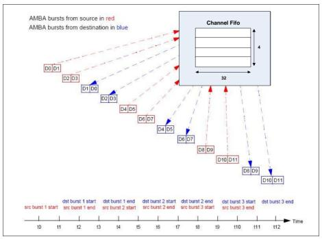
Figure 5-12 Breakdown of Block Transfer where max abrst = 2, Case 2
