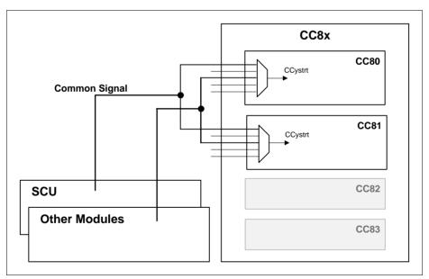
Figure 23-6 Start multiple timers synchronously
