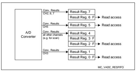
Figure 19-17 Result FIFO Buffers
