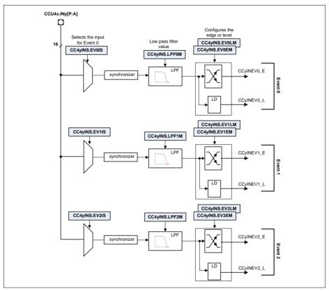
Figure 22-3 Slice input selector diagram
