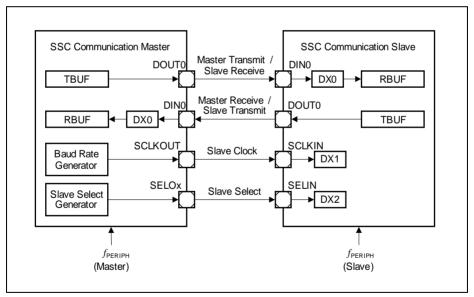
Figure 17-35 SSC Signals for Standard Full-Duplex Communication
