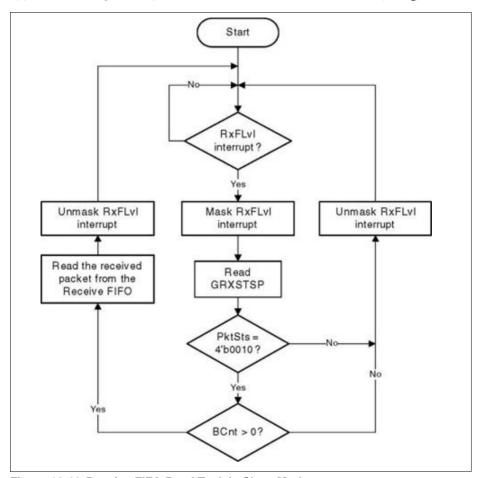
Figure 16-10 Receive FIFO Read Task in Slave Mode
