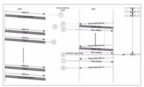
Figure 16-60 Isochronous IN Transfers
