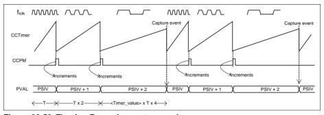
Figure 22-59 Floating Prescaler capture mode usage
