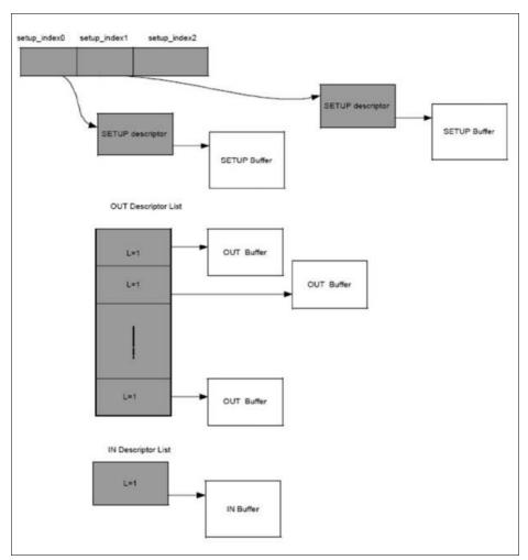
Figure 16-39 Descriptor Lists for Handling Control Transfers
