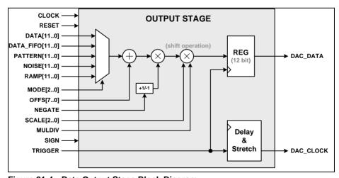
Figure 21-4 Data Output Stage Block Diagram
