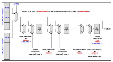
Figure 21-8 Data Handling for the FIFO Buffer
