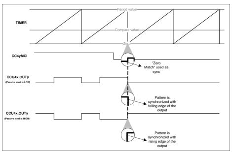
Figure 22-36 Multi channel pattern synchronization
