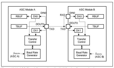
Figure 17-30 ASC Signal Connections for Half-Duplex Communication
