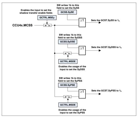
Figure 22-11 Usage of the CCU4x.MCSS input
