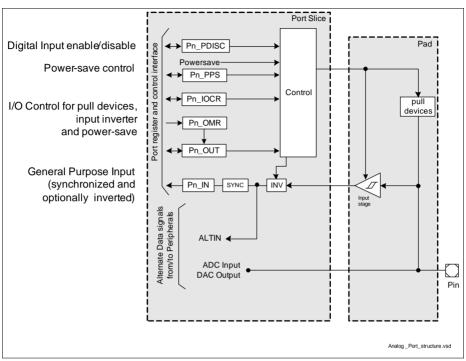
Figure 25-3 Analog Port Structure
