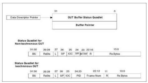
Figure 16-37 Out Data Memory Structure
