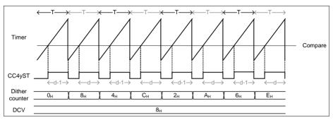
Figure 22-48 Dither timing diagram in edge aligned - CC4yTC.DITHE = 10<sub>B</sub>
