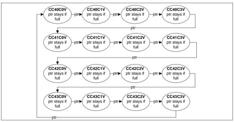
Figure 22-65 Extended Capture Read back
