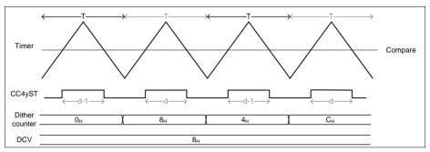
Figure 22-51 Dither timing diagram in center aligned - CC4yTC.DITHE = 10<sub>B</sub>
