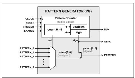
Figure 21-5 Pattern Generator Block Diagram
