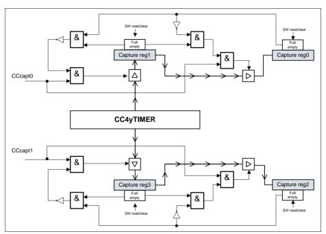
Figure 22-26 Slice capture logic
