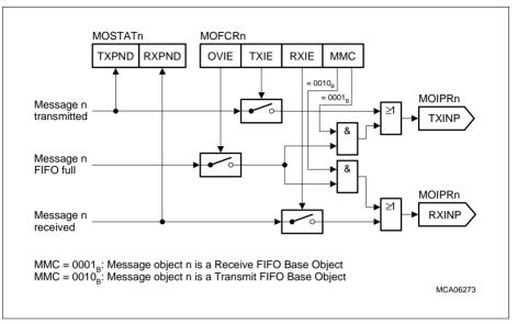
Figure 18-15 Message Interrupt Request Routing
