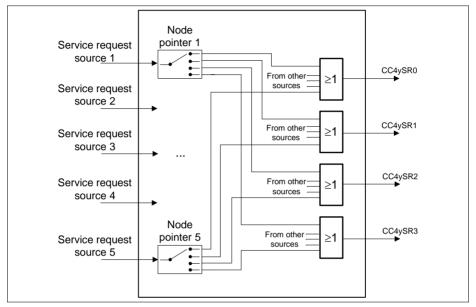
Figure 22-68 Slice Interrupt Node Pointer overview
