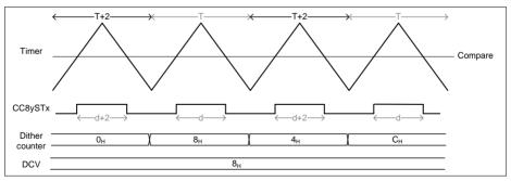
Figure 23-68 Dither timing diagram in center aligned - CC8yTC.DITHE = 01<sub>B</sub>
