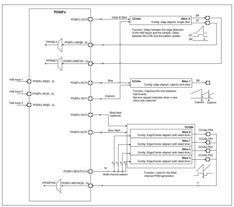
Figure 24-15 Hall Sensor Mode usage - profile 1
