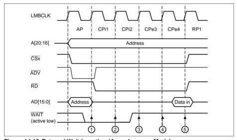
Figure 14-19 External Wait Insertion (Asynchronous Mode)
