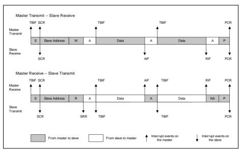
Figure 17-56 Interrupt Events on Data Transfers
