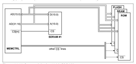
Figure 14-27 Connectivity for 16-bit SDRAM
