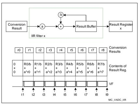
Figure 19-21 IIR Filter Structure
