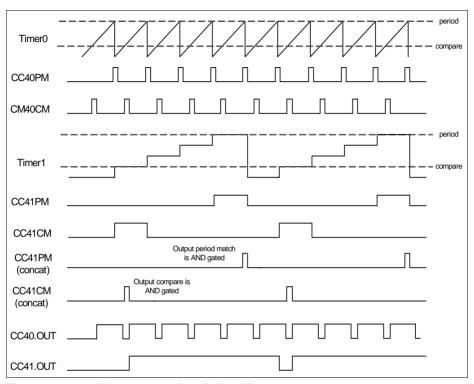
Figure 22-43 32 bit concatenation timing diagram
