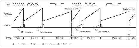
Figure 23-77 Floating Prescaler capture mode usage
