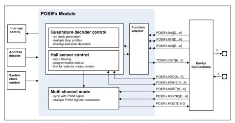
Figure 24-1 POSIF block diagram
