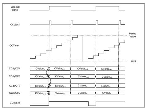
Figure 23-42 External Capture - CC8yTC.SCE = 1<sub>B</sub>
