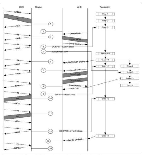
Figure 16-46 Extra IN Tokens During Control Read Data Phase
