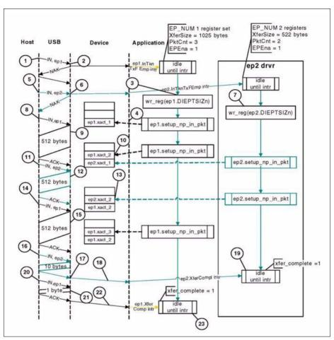
Figure 16-27 Slave Mode Bulk IN Two-Endpoint Transfer
