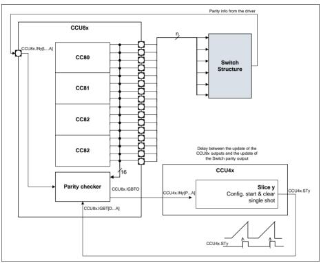
Figure 23-85 Parity Checker connections
