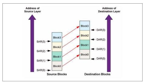
Figure 5-27 Multi-Block with Linked Address for Source and Destination Where SAR and DAR Between Successive Blocks are Contiguous
