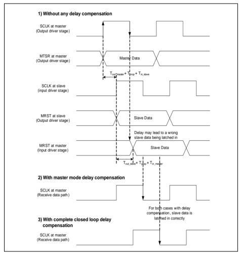
Figure 17-46 SSC Closed-loop Delay Timing Waveform
