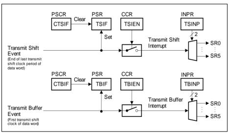
Figure 17-7 Transmit Events and Interrupts
