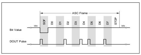
Figure 17-34 Pulse Output Example
