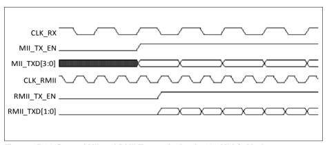
Figure 15-21 Start of MII and RMII Transmission in 100 Mbit/s Mode
