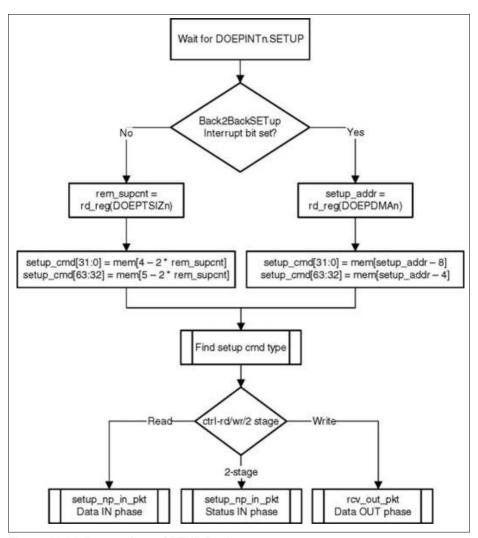
Figure 16-33 Processing a SETUP Packet
