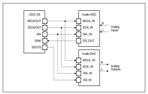
Figure 17-60 Connection of External Audio Devices
