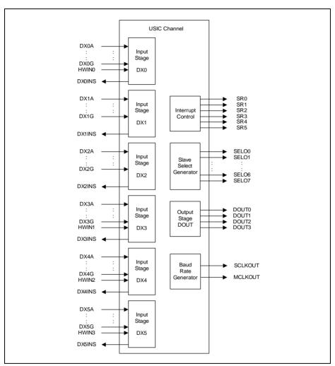
Figure 17-66 USIC Channel I/O Lines
