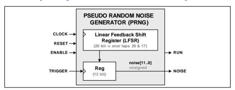
Figure 21-6 Noise Generator Block Diagram
