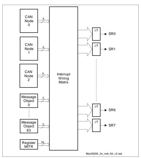
Figure 18-21 Interrupt Compressor
