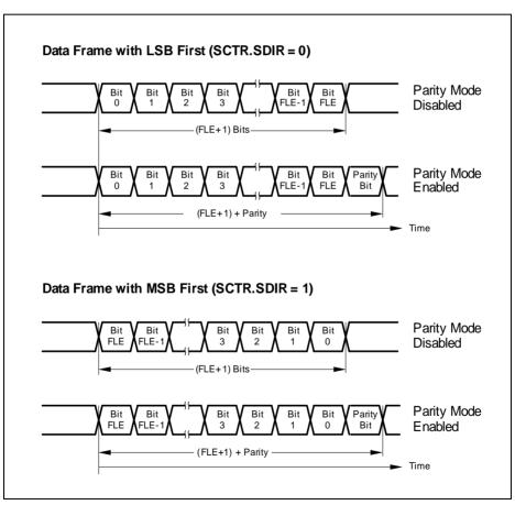
Figure 17-41 Data Frames without/with Parity
