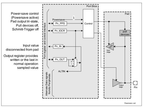
Figure 25-2 Port Pin in Power Save State
