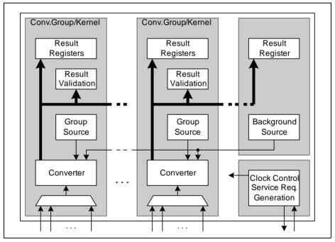
Figure 19-1 ADC Structure Overview
