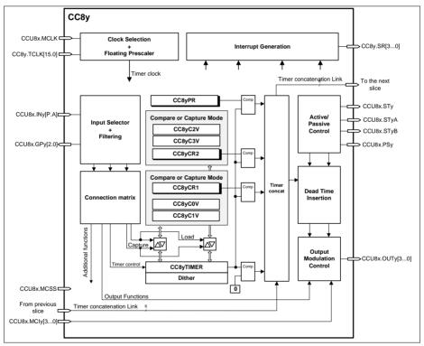
Figure 23-2 CCU8 slice block diagram
