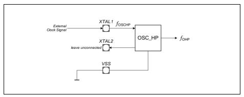
Figure 11-20 External Clock Input Mode for the High-Precision Oscillator
