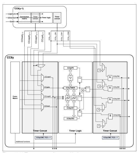
Figure 23-60 Timer concatenation control logic
