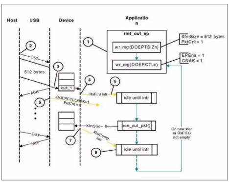
Figure 16-28 Slave Mode Bulk OUT Transaction
