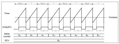
Figure 23-65 Dither timing diagram in edge aligned - CC8yTC.DITHE = 01<sub>B</sub>
