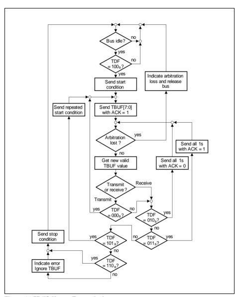
Figure 17-55 IIC Master Transmission
