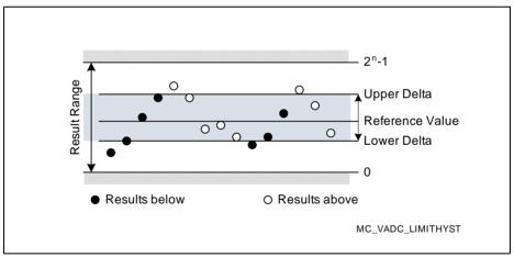
Figure 19-12 Result Monitoring through Compare with Hysteresis
