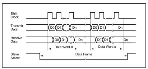
Figure 17-36 4-Wire SSC Standard Communication Signals
