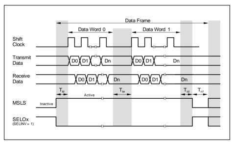
Figure 17-44 MSLS Generation in SSC Master Mode
