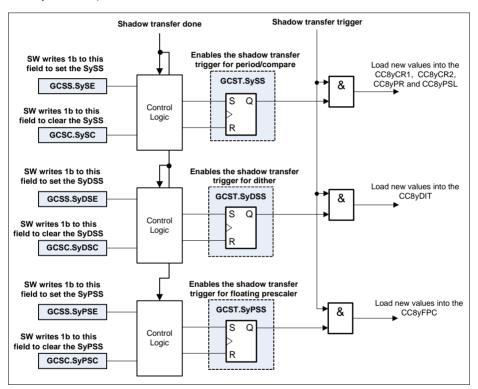
Figure 23-9 Shadow transfer enable logic
