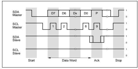
Figure 17-50 IIC Frame Example (simplified)
