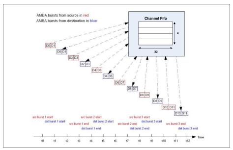
Figure 5-10 Breakdown of Block Transfer where max\_abrst = 2, Case 1
