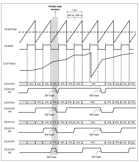
Figure 22-63 Three Capture profiles - CC4yTC.SCE = 1<sub>B</sub>
