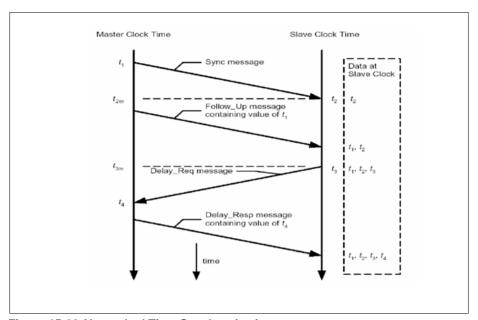
Figure 15-26 Networked Time Synchronization
