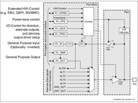
Figure 25-1 General Structure of a digital Port Pin
