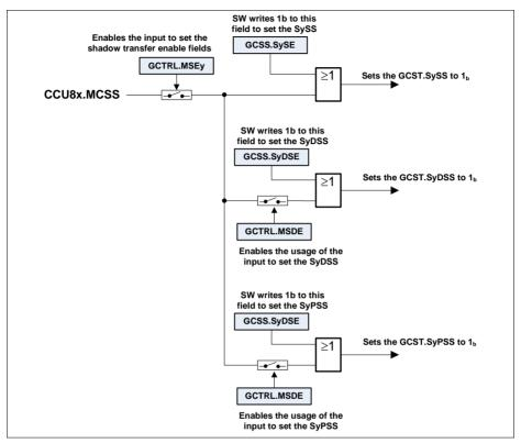
Figure 23-11 Usage of the CCU8x.MCSS input
