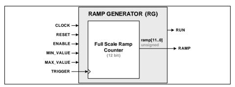
Figure 21-7 Ramp Generator Block Diagram
