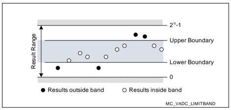
Figure 20-9 Result Monitoring through Limit Checking
