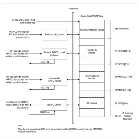
Figure 16-70 Host Mode FIFO Address Mapping
