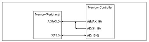
Figure 14-9 Connection of a 16-bit non-Multiplexed Device to Memory Controller
