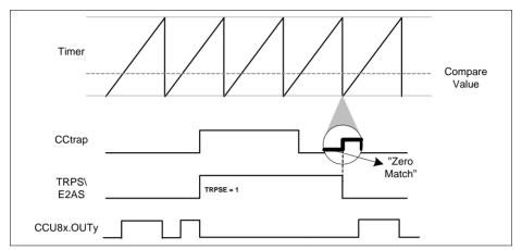
Figure 23-49 Trap synchronization with the PWM signal
