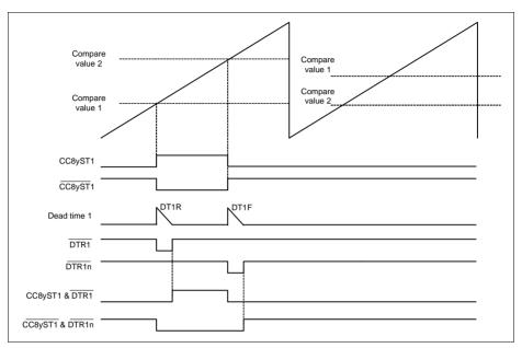
Figure 23-25 Edge Aligned - Asymmetric PWM timing, CC8yCR1.CR1 > CC8yCR2.CR2
