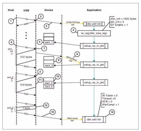
Figure 16-26 Slave Mode Bulk IN Transfer (Pipelined Transaction
