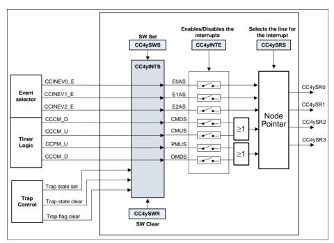
Figure 22-67 Slice interrupt structure overview
