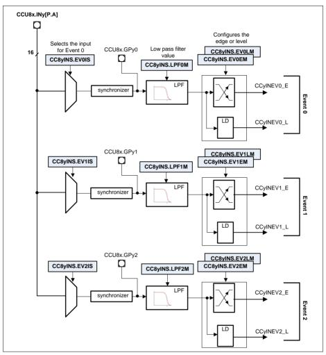
Figure 23-3 Slice input selector diagram
