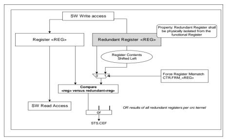
Figure 6-4 Register monitoring scheme
