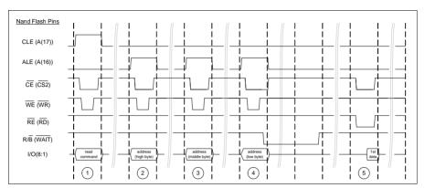
Figure 14-22 Example of an Memory Controller Nand Flash access sequence (read)
