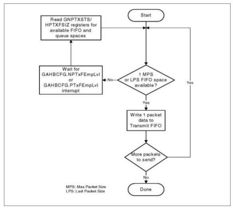
Figure 16-9 Transmit FIFO Write Task in Slave Mode
