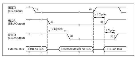
Figure 14-12 Arbitration Sequence with the EBU in Arbiter Mode
