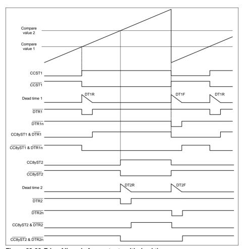
Figure 23-22 Edge Aligned - four outputs with dead time
