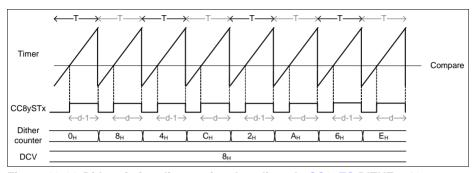
Figure 23-66 Dither timing diagram in edge aligned - CC8yTC.DITHE = 10<sub>B</sub>
