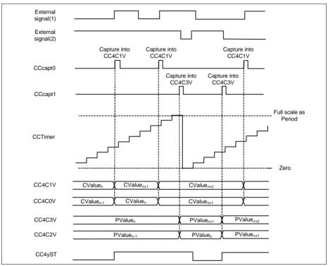
Figure 22-25 External capture - CC4yCMC.CAP0S != 00<sub>B</sub>, CC4yCMC.CAP1S != 00<sub>B</sub>
