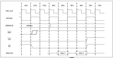
Figure 14-25 Terminating a Burst by de-asserting CS
