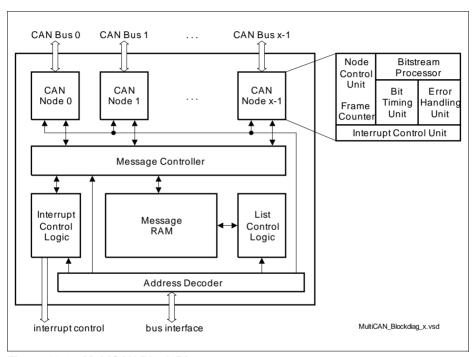
Figure 18-6 MultiCAN Block Diagram
