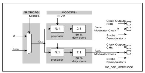
Figure 20-4 Modulator Clock Configuration
