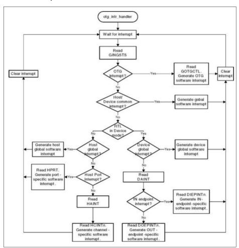
Figure 16-72 Core Interrupt Handler
