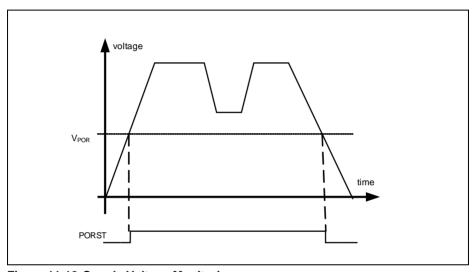
Figure 11-12 Supply Voltage Monitoring
