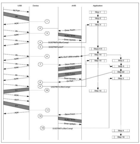
Figure 16-50 Premature Status Phase During Control Read
