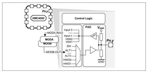
Figure 25-4 Simplified Port Structure
