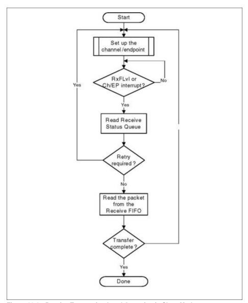
Figure 16-6 Receive Transaction-Level Operation in Slave Mode
