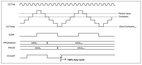
Figure 22-56 PWM with 100% duty cycle - Center Aligned Mode
