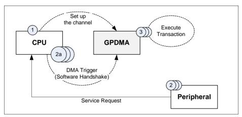
Figure 5-5 Software Handshaking Interface
