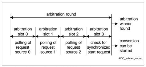
Figure 19-8 Arbitration Round with 4 Arbitration Slots
