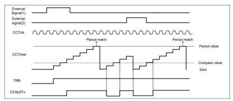
Figure 23-31 Start (as start)/ stop (as flush) - CC8yTC.STRM =  $0_B$ , CC8yTC.ENDM =  $01_R$
