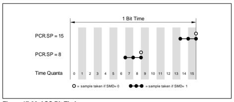
Figure 17-32 ASC Bit Timing
