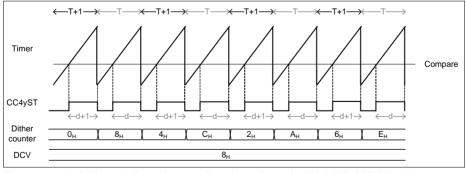
Figure 22-47 Dither timing diagram in edge aligned - CC4yTC.DITHE = 01<sub>B</sub>
