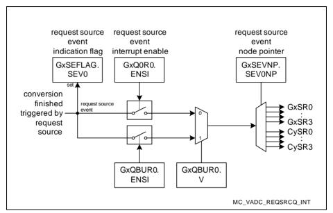
Figure 19-6 Interrupt Generation of a Queued Request Source
