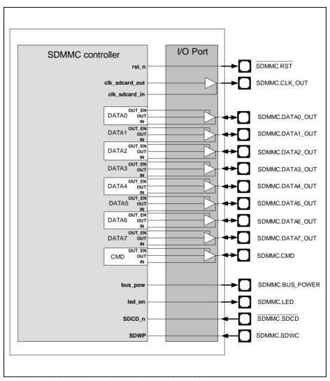
Figure 13-4 External Pin Connections of SDMMC
