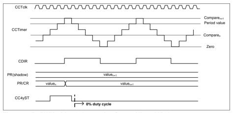
Figure 22-58 PWM with 0% duty cycle - Center Aligned Mode
