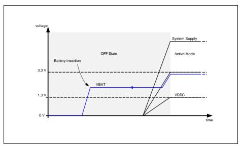
Figure 11-11 Initial power-up sequence
