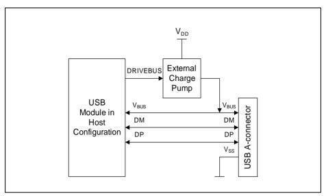
Figure 16-3 USB Host Connections
