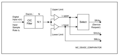
Figure 20-10 Comparator Structure
