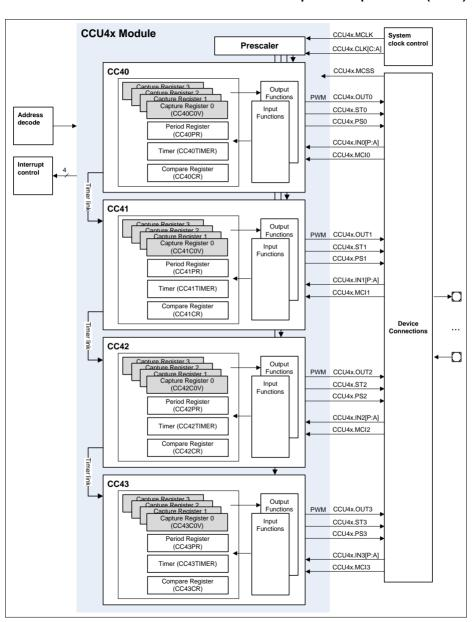
Figure 22-1 CCU4 block diagram
