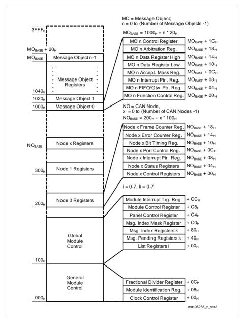
Figure 18-26 MultiCAN Module Register Map
