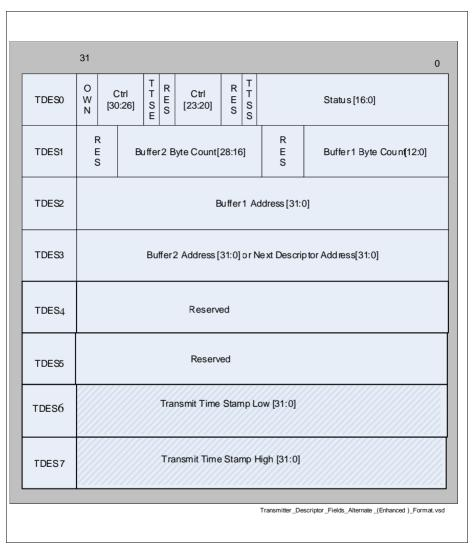
Figure 15-11 Transmitter Descriptor Fields - Alternate (Enhanced) Format
