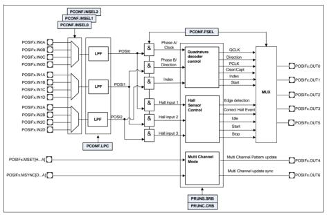
Figure 24-2 Function selector diagram
