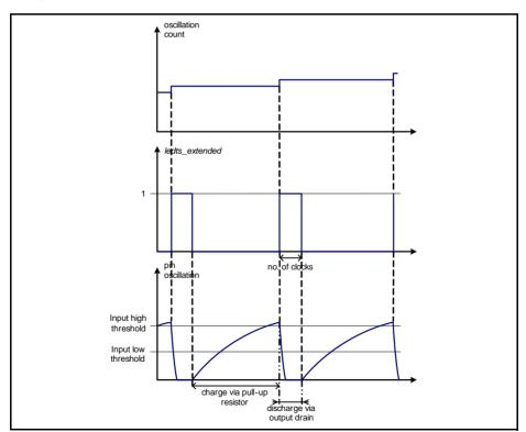
Figure 12-7 Pin-Low-Level Extension Function
