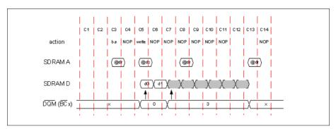
Figure 14-29 Short Burst Write Access through Data Masking
