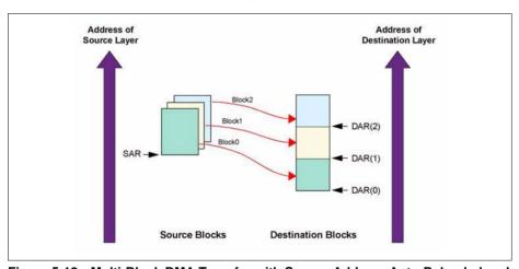
Figure 5-18 Multi-Block DMA Transfer with Source Address Auto-Reloaded and Contiguous Destination Address
