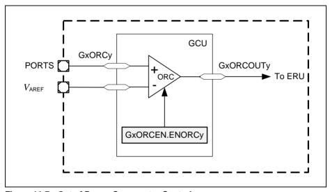
Figure 11-7 Out of Range Comparator Control
