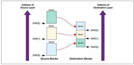
Figure 5-24 Multi-Block DMA Transfer with Linked List Source Address and Contiguous Destination Address
