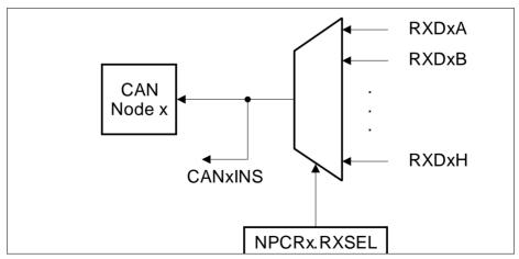
Figure 18-28 CAN Module Receive Input Selection
