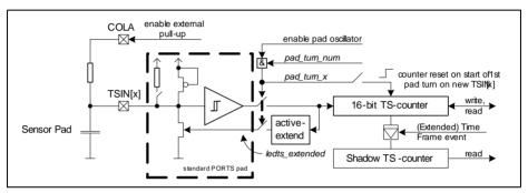
Figure 12-5 Touch-Sense Oscillator Control Circuit
