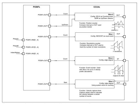
Figure 24-17 Quadrature Decoder Mode usage - profile 1
