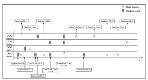
Figure 22-66 Extended Capture Access Example
