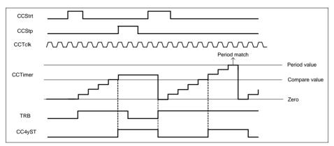
Figure 22-18 Start (as flush and start)/ stop (as stop) - CC4yTC.STRM = 1<sub>B</sub>, CC4yTC.ENDM = 00<sub>R</sub>
