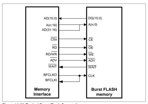
Figure 14-23 Typical Burst Flash Connection
