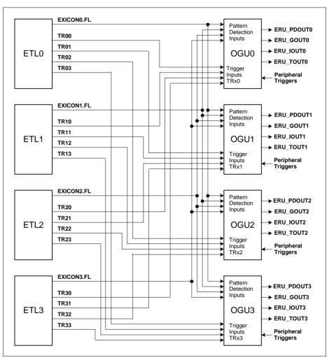
Figure 4-7 ERU Cross Connect Matrix
