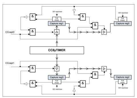
Figure 23-41 Slice capture logic
