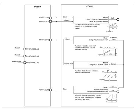
Figure 24-21 Quadrature Decoder Mode usage - profile 4
