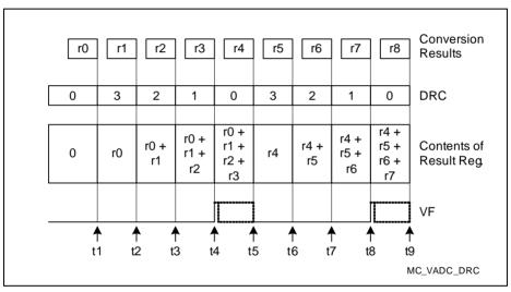
Figure 19-18 Standard Data Reduction Filter
