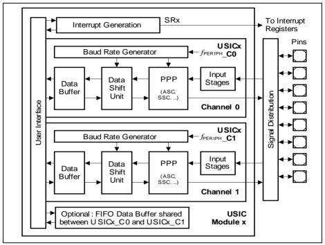
Figure 17-1 USIC Module/Channel Structure
