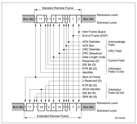
Figure 18-3 CAN Remote Frame
