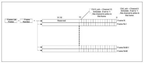
Figure 16-20 Frame List for Periodic Channels
