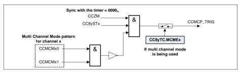
Figure 23-20 Dead Time trigger with the Multi Channel pattern
