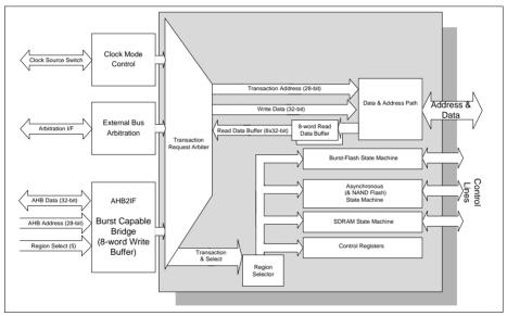
Figure 14-3 Memory Controller Block Diagram
