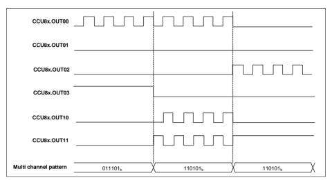
Figure 23-53 Multi Channel mode for multiple Timer Slices
