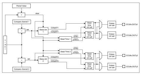
Figure 23-21 Edge Aligned with two independent channels scheme
