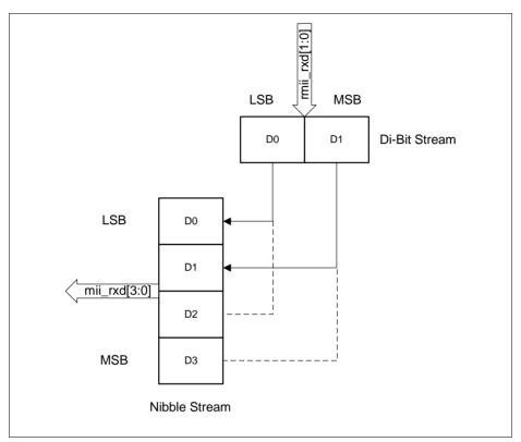
Figure 15-25 Receive Bit Ordering
