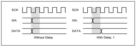
Figure 17-59 Transfer Delay for IIS
