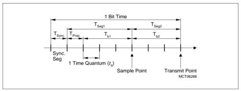
Figure 18-8 CAN Bus Bit Timing Standard
