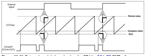
Figure 22-29 External modulation clearing the ST bit - CC4yTC.EMT =  $0_B$
