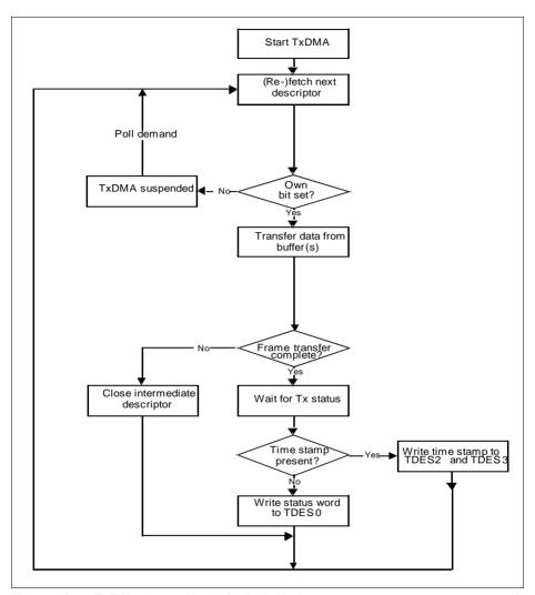
Figure 15-3 TxDMA Operation in Default Mode
