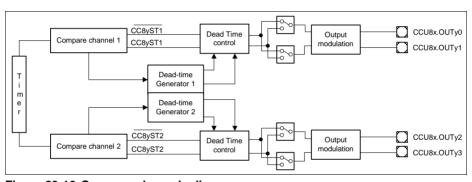
Figure 23-16 Compare channels diagram
