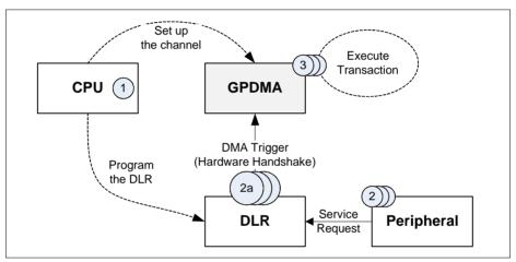
Figure 5-4 Hardware Handshaking Interface
