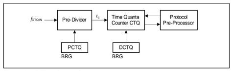
Figure 17-15 Time Quanta Counter
