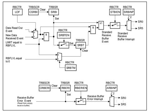
Figure 17-25 Receiver Buffer Events in Filling Level Mode
