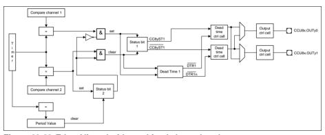
Figure 23-23 Edge Aligned with combined channels scheme
