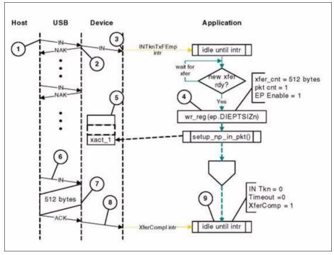
Figure 16-25 Slave Mode Bulk IN Transaction
