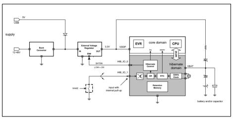
Figure 11-14 System Level Power Control example - externally controlled with two pins
