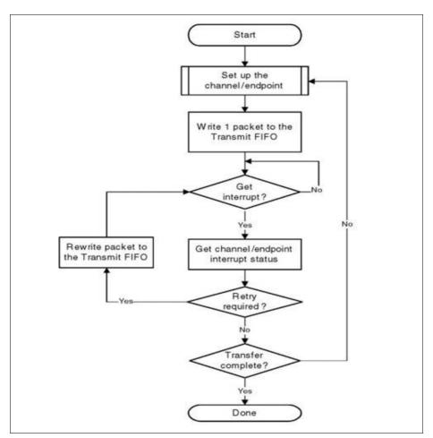
Figure 16-5 Transmit Transaction-Level Operation in Slave Mode
