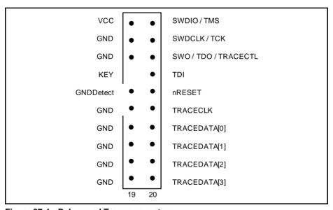
Figure 27-4 Debug and Trace connector
