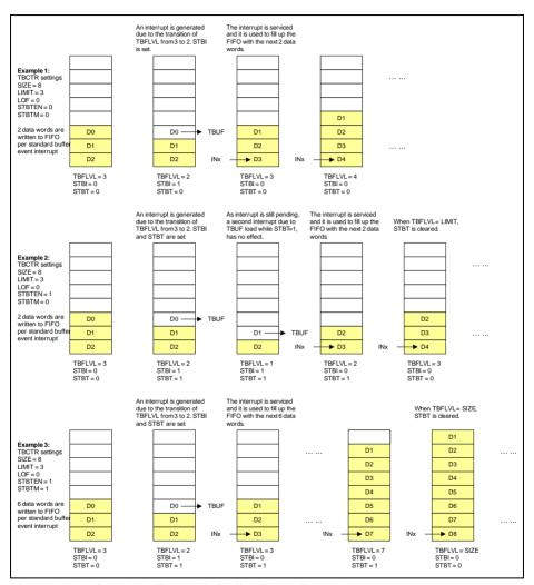
Figure 17-22 Standard Transmit Buffer Event Examples
