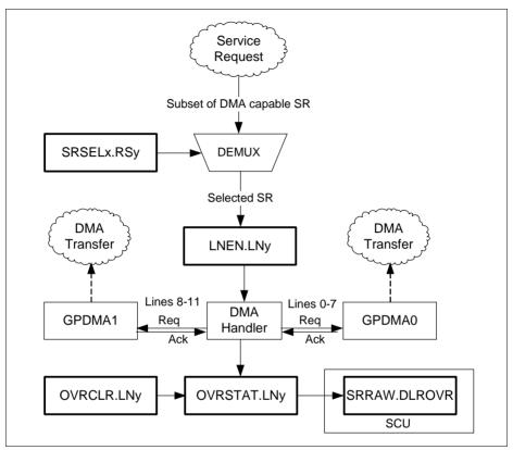
Figure 4-3 DMA Line Handler
