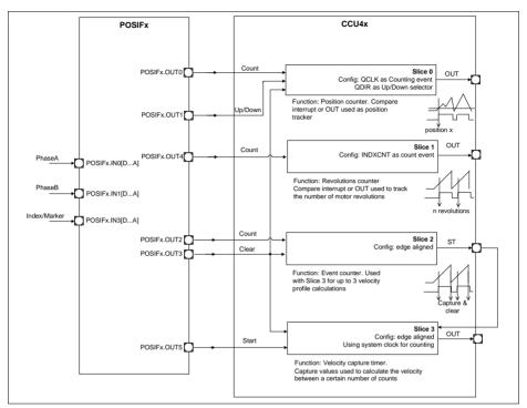
Figure 24-19 Quadrature Decoder Mode usage - profile 3
