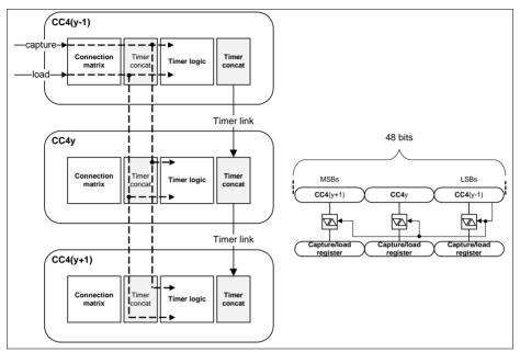
Figure 22-42 Capture/Load Timer Concatenation
