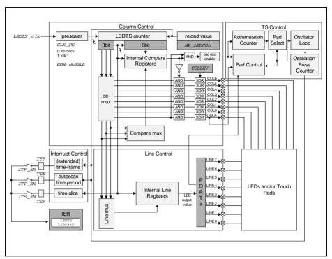
Figure 12-1 LEDTS Block Diagram
