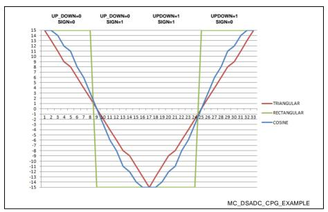
Figure 20-12 Example Pattern/Waveform Outputs
