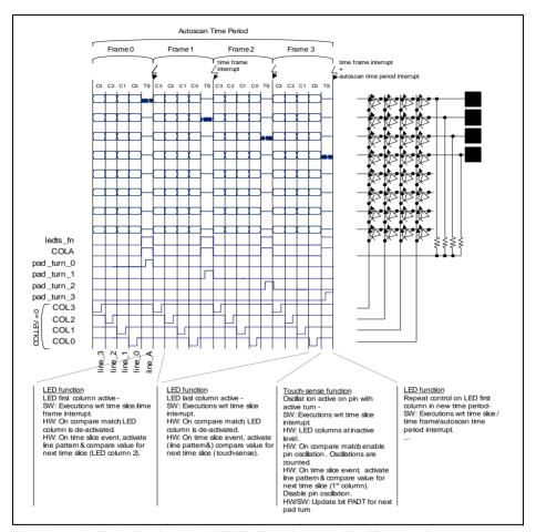
Figure 12-2 Time-Multiplexed LEDTS Functions on Pin (Example)
