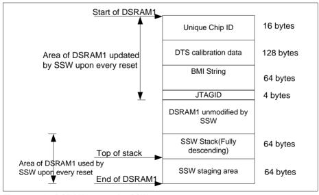
Figure 26-1 DSRAM1 usage by SSW
