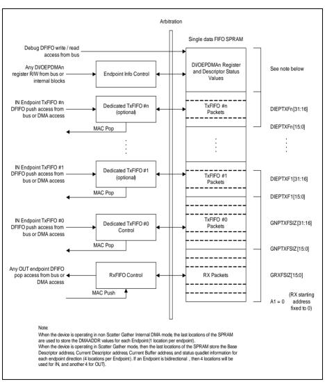
Figure 16-69 Device Mode FIFO Address Mapping
