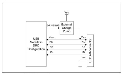
Figure 16-2 OTG DRD Connections
