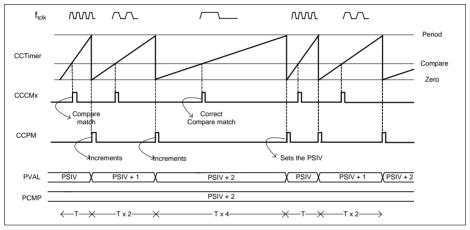
Figure 23-78 Floating Prescaler compare mode usage - Edge Aligned
