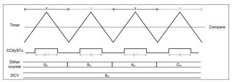
Figure 23-69 Dither timing diagram in center aligned - CC8yTC.DITHE = 10<sub>B</sub>
