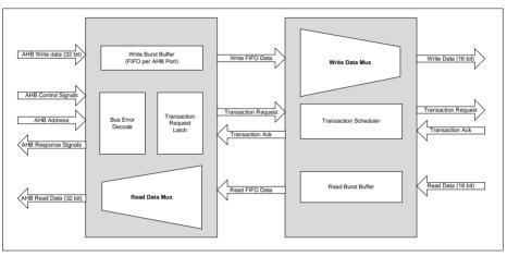
Figure 14-4 AHB Bridge Block Diagram
