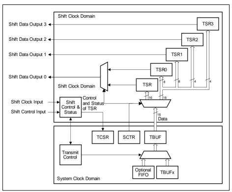
Figure 17-17 Transmit Data Path
