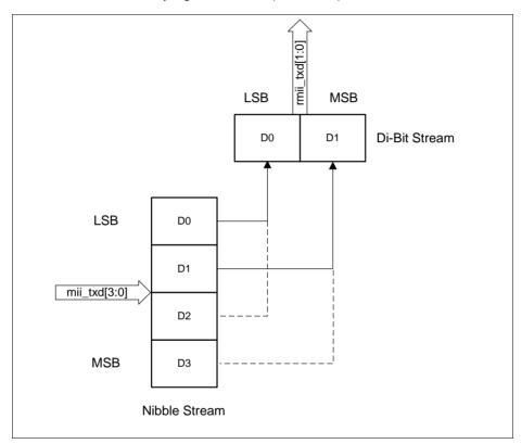
Figure 15-20 Transmission Bit Ordering
