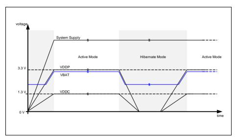
Figure 11-10 Hibernate controlled with external voltage regulator
