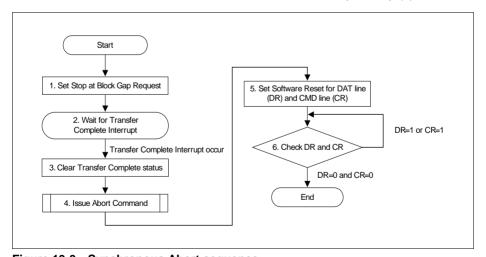
Figure 13-3 Synchronous Abort sequence
