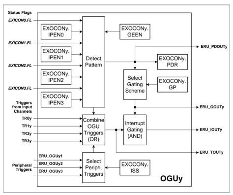
Figure 4-8 Output Gating Unit for Output Channel y
