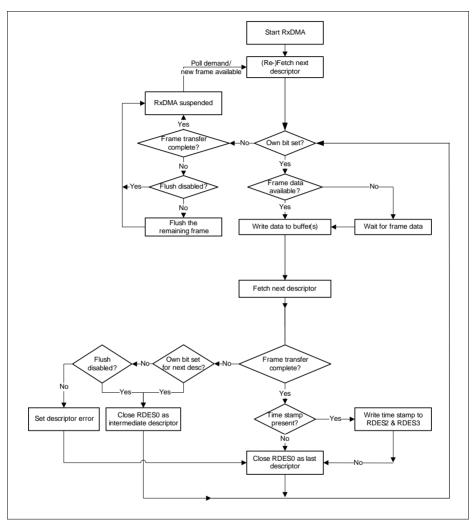
Figure 15-5 Receive DMA Operation
