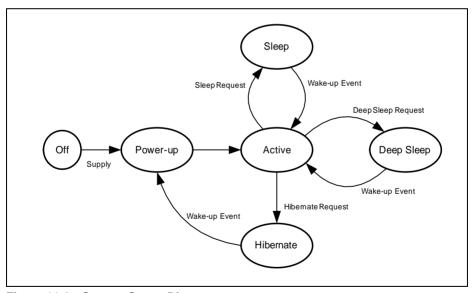
Figure 11-8 System States Diagram
