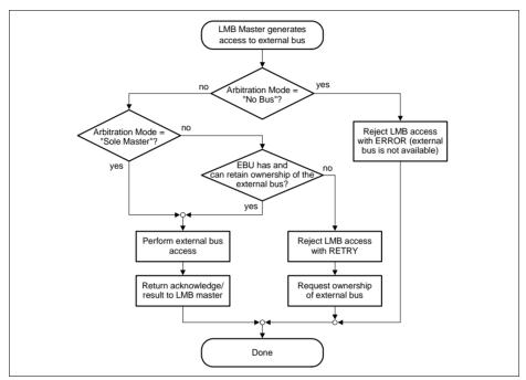
Figure 14-16 EBU Reaction to AHB to External Bus Access
