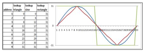
Figure 21-9 Example 5-bit Patterns and their corresponding Waveform Output
