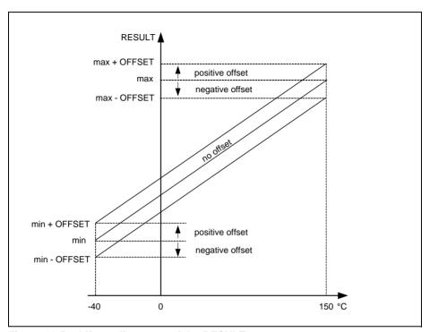
Figure 11-5 Offset adjustment of the RESULT curve
