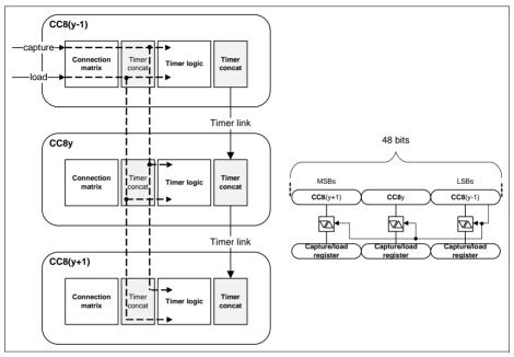
Figure 23-58 Capture/Load Timer Concatenation
