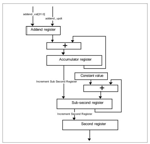
Figure 15-28 System Time Update Using Fine Method
