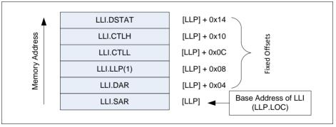
Figure 5-17 Mapping of Block Descriptor (LLI) in Memory to Channel Registers When CFG.SS UPD EN = 0
