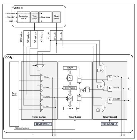
Figure 22-44 Timer concatenation control logic
