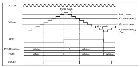
Figure 22-13 Center aligned mode, CC4yTC.TCM = 1<sub>B</sub>
