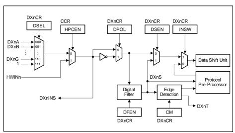
Figure 17-10 Input Conditioning for DX0 and DX[5:3]
