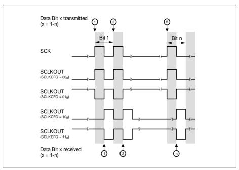
Figure 17-39 SCLKOUT Configuration in SSC Master Mode
