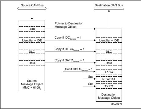
Figure 18-20 Gateway Transfer from Source to Destination
