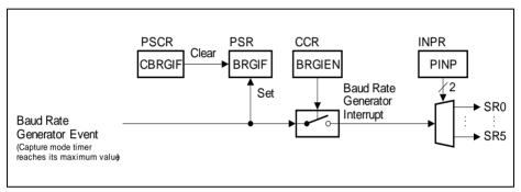
Figure 17-9 Baud Rate Generator Event and Interrupt
