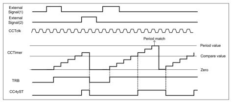
Figure 22-19 Start (as start)/ stop (as flush and stop) - CC4yTC.STRM = 0<sub>B</sub>, CC4yTC.ENDM = 10<sub>B</sub>
