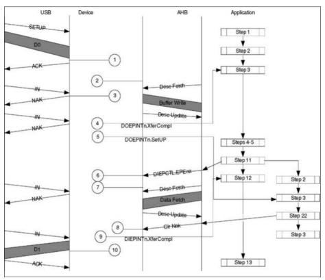
Figure 16-42 Two-Stage Control Transfer
