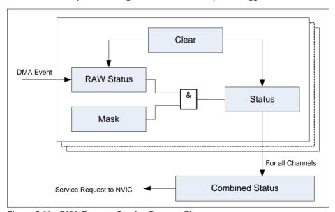
Figure 5-29 DMA Event to Service Request Flow
