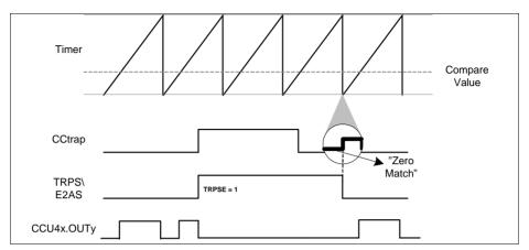
Figure 22-34 Trap synchronization with the PWM signal, CC4yTC.TRPSE = 1<sub>B</sub>
