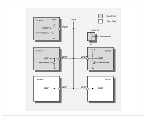
Figure 11-26 System Level Power On Reset Control
