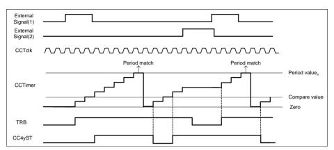
Figure 22-16 Start (as start)/ stop (as stop) -  $CC4yTC.STRM = 0_B$ ,  $CC4yTC.ENDM = 00_B$
