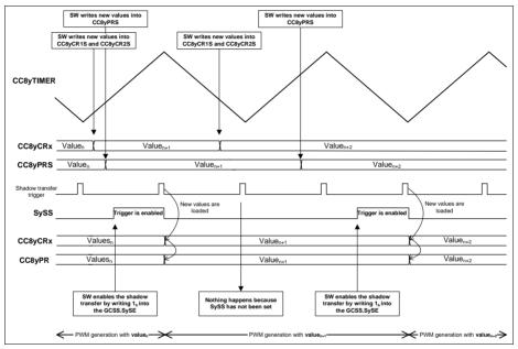
Figure 23-10 Shadow transfer timing example - center aligned mode
