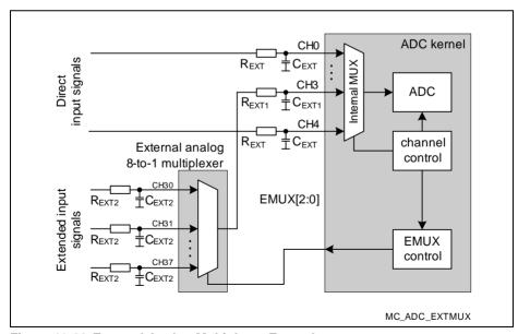
Figure 19-28 External Analog Multiplexer Example
