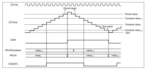
Figure 23-13 Center aligned mode, CC8yTC.TCM = 1<sub>B</sub>
