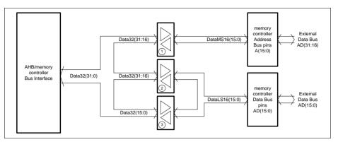
Figure 14-10 AHB to External Bus Data Re-Alignment
