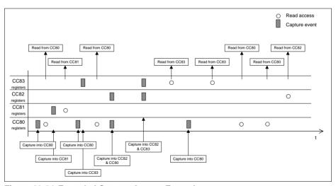
Figure 23-84 Extended Capture Access Example
