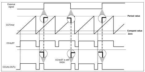
Figure 22-31 External modulation gating the output - CC4yTC.EMT = 1<sub>B</sub>
