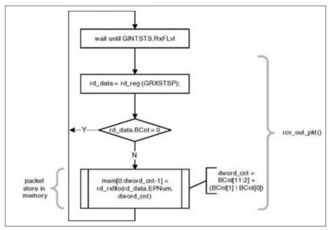
Figure 16-23 Receive FIFO Packet Read in Slave Mode
