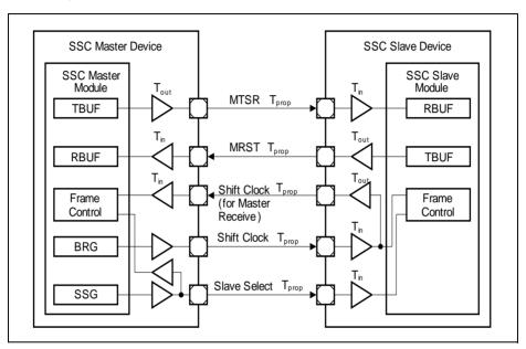
Figure 17-48 SSC Complete Closed-loop Delay Compensation
