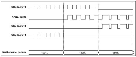
Figure 22-37 Multi Channel mode for multiple Timer Slices
