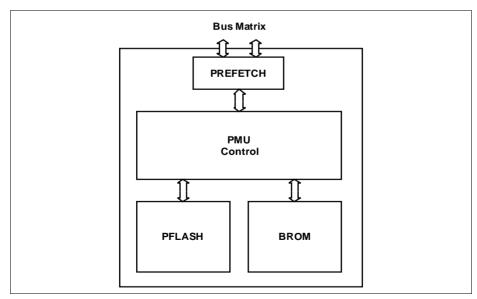
Figure 8-1 PMU Block Diagram
