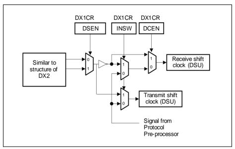
Figure 17-12 Delay Compensation Enable in DX1
