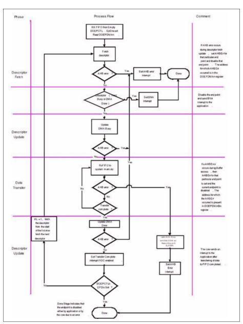
Figure 16-61 Isochronous OUT Descriptor/Data Buffer Processing
