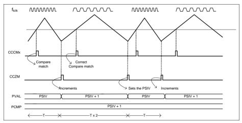
Figure 23-79 Floating Prescaler compare mode usage - Center Aligned
