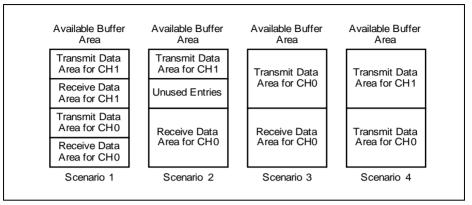
Figure 17-21 FIFO Buffer Partitioning
