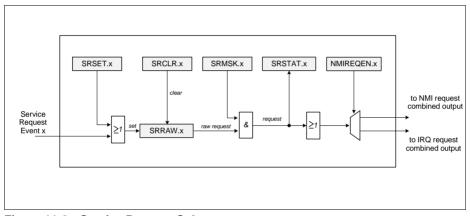
Figure 11-2 Service Request Subsystem
