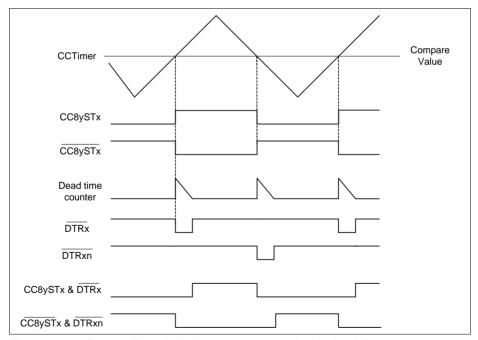
Figure 23-27 Center aligned - Independent channel with dead time
