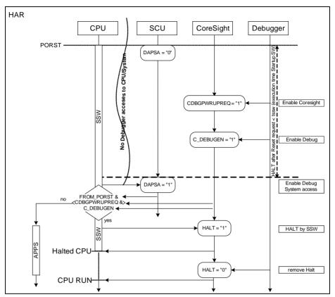
Figure 27-2 HAR - Halt After Reset
