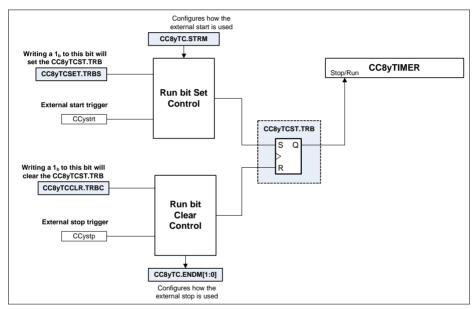
Figure 23-5 Timer start/stop control diagram
