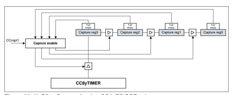
Figure 23-43 Slice Capture Logic -  $CC8yTC.SCE = 1_B$
