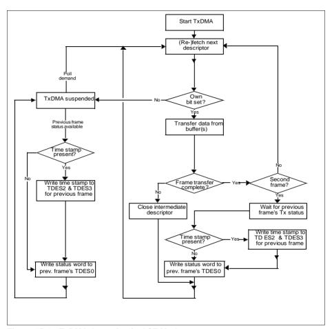
Figure 15-4 TxDMA Operation in OSF Mode
