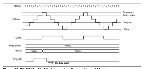
Figure 23-76 PWM with 0% duty cycle - Center Aligned Mode
