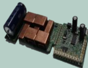
Power Tool KIT using XMC1302 1 kW/20 V DC BLDC Motor Control
