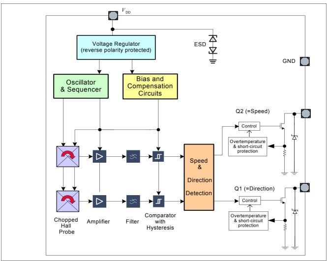
Figure 2 Block diagram of the TLE4966V-1K
