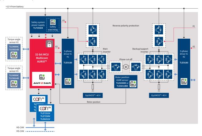
Infineon EPS system solution for high-availability autonomous drive systems L0–L3
