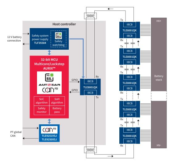
The battery management system controls the battery state during charging and discharging. Intelligent functionality is needed to extend the battery lifetime, which has a considerable impact on the total cost of ownership. The State of Health (SoH), State of Charge (SoC) and Depth of Discharge (DoD) of the battery is permanently monitored.
