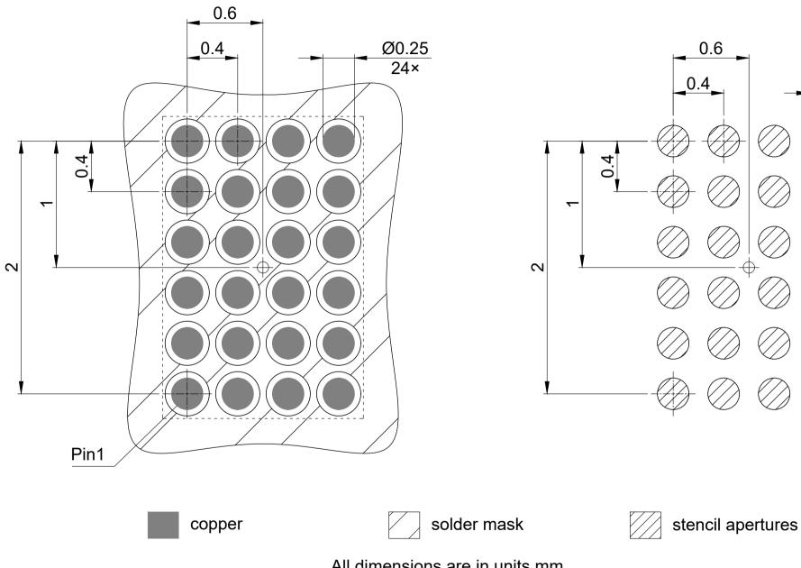
All dimensions are in units mm All pads are non-solder mask defined Ø0.25
