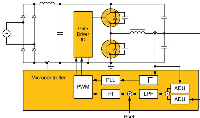
Figure 2: Half-Bridge Inverter that is used in Half-Bridge based induction cooking hobs
