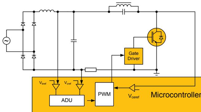
Figure 1: Quasi-Resonant Inverter (single-switch) that is used for Single-Ended induction cooking hobs
