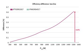
Performance gain of 0.6 percent full load efficiency gain TOLL versus TO-247 due to lower  $R_{\text{DS(on)}}$  from TOLL and 4pin Kelvin source capability.
