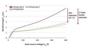
CoolMOS<sup>TM</sup> G7 technology improves again over previous best 650 V CoolMOS<sup>TM</sup> C7 performance in  $E_{oss}$ , a key value in hard switching topologies such as PFC.
