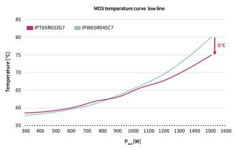
5°C lower temperature seen for TOLL as higher efficiency means less thermal losses produced.
