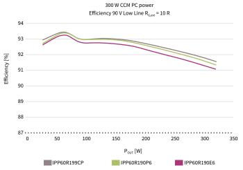
This plug and play measurement shows the benefit of CoolMOS™ P6 in comparison to CoolMOS™ E6 and CoolMOS™ CP. In this 300 W continuous conduction mode (CCM) PC power, CCM operates after output power until 70 W or higher otherwise it works in DCM. Even in this light load condition, which is not a one to one comparison,
