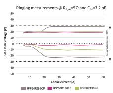
The  $V_{GS}$  peak is measured in a typical PFC stage with 5  $\Omega$  R<sub>G,ext</sub> and exhibiting 7.2 pF capacitive coupling between gate and drain emulating the parasitic capacitance of the PCB. In the measurement, CoolMOS<sup>TM</sup> P6 shows very good gate switching waveform with reduced  $Q_G$  and internal R<sub>G</sub>. The slight increase in magnitude of oscillations in CoolMOS<sup>TM</sup> P6 over CoolMOS<sup>TM</sup> E6 is expected due to its faster switching characteristic.
