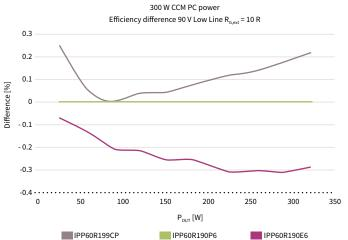
CoolMOS<sup>TM</sup> P6 has a slight efficiency improvement. When the output power over 70 W CCM is operated, the efficiency improvement of CoolMOS<sup>TM</sup> P6 is visible in the range of 0.2% till 0.3% in full-load, compared with that of CoolMOS<sup>TM</sup> E6. This efficiency benefit is due to  $Q_c$  reduction and relatively high  $V_{th}$  values.
