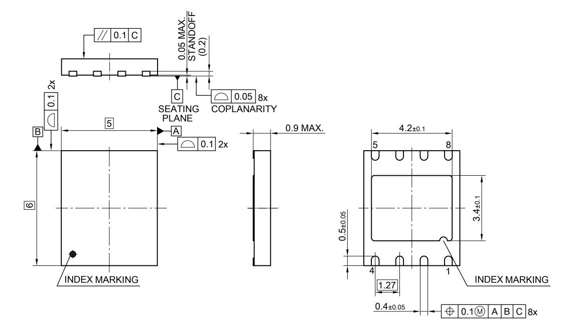
ALL DIMENSIONS ARE IN UNITS MM THE DRAWING IS IN COMPLIANCE WITH ISO 128 & PROJECTION METHOD 1 [
