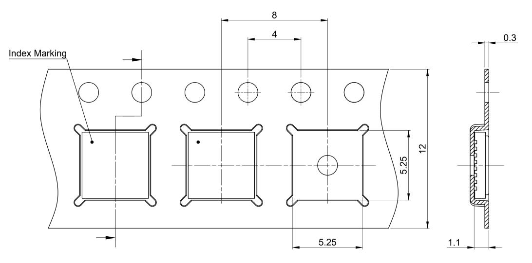
All dimensions are in units mm The drawing is in compliance with ISO 128-30, Projection Method 1 [ $-\Box \oplus$ ]
