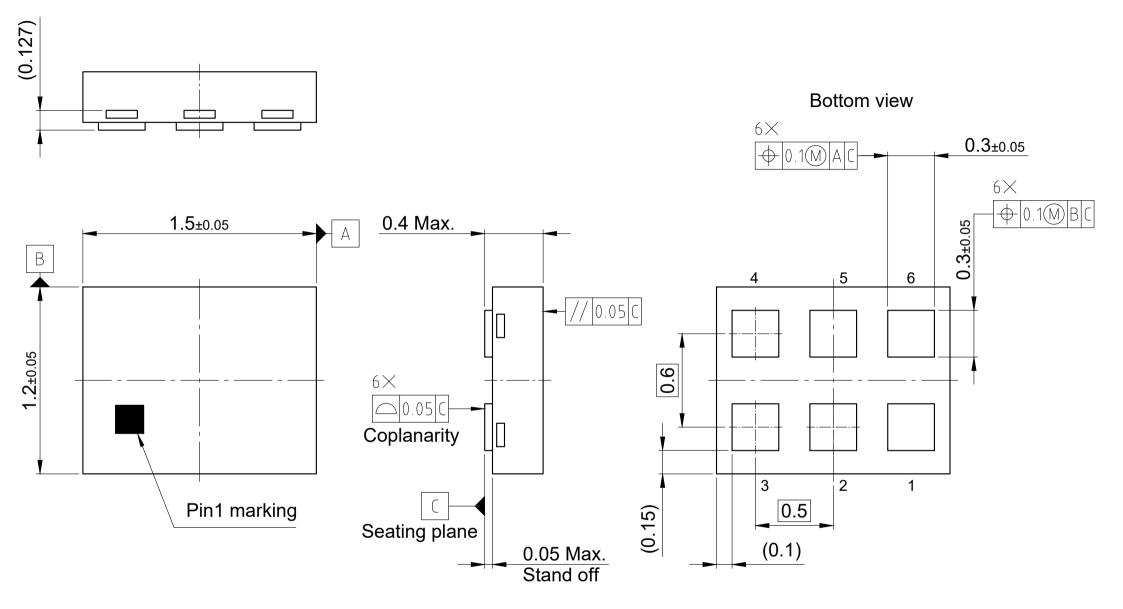
All dimensions are in units mm The drawing is in compliance with ISO 128-30, Projection Method 1 [ $-\Box \oplus$ ]
