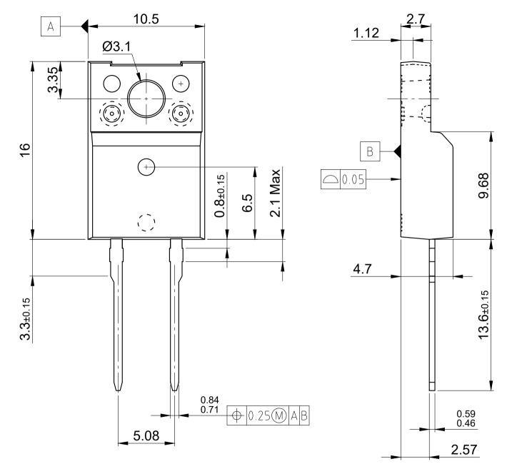
All dimensions do not include mold flash or protrusions
