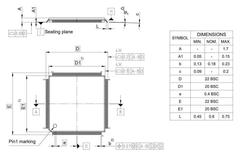
Dimensions D1 and E1 do not include mold protrusion.allowable protrusion is 0.25mm per side.
