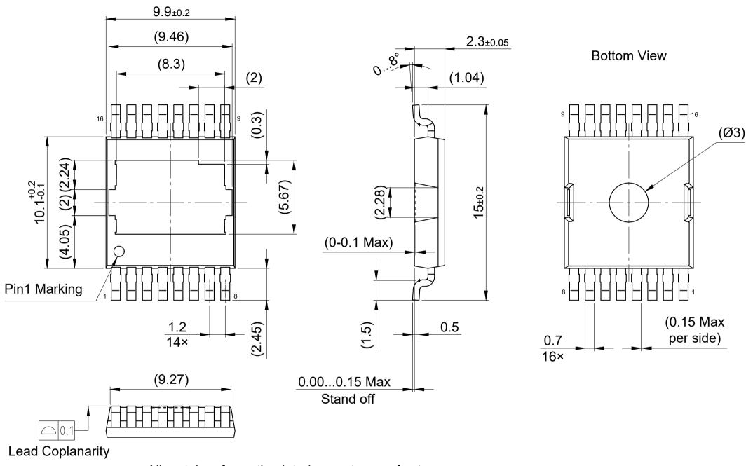
All metal surfaces tin plated except area of cut All dimensions are in units mm The drawing is in compliance with ISO 128-30, Projection Method 1 [] ] Drawing according to ISO 8015, general tolerances ISO 2768-mK
