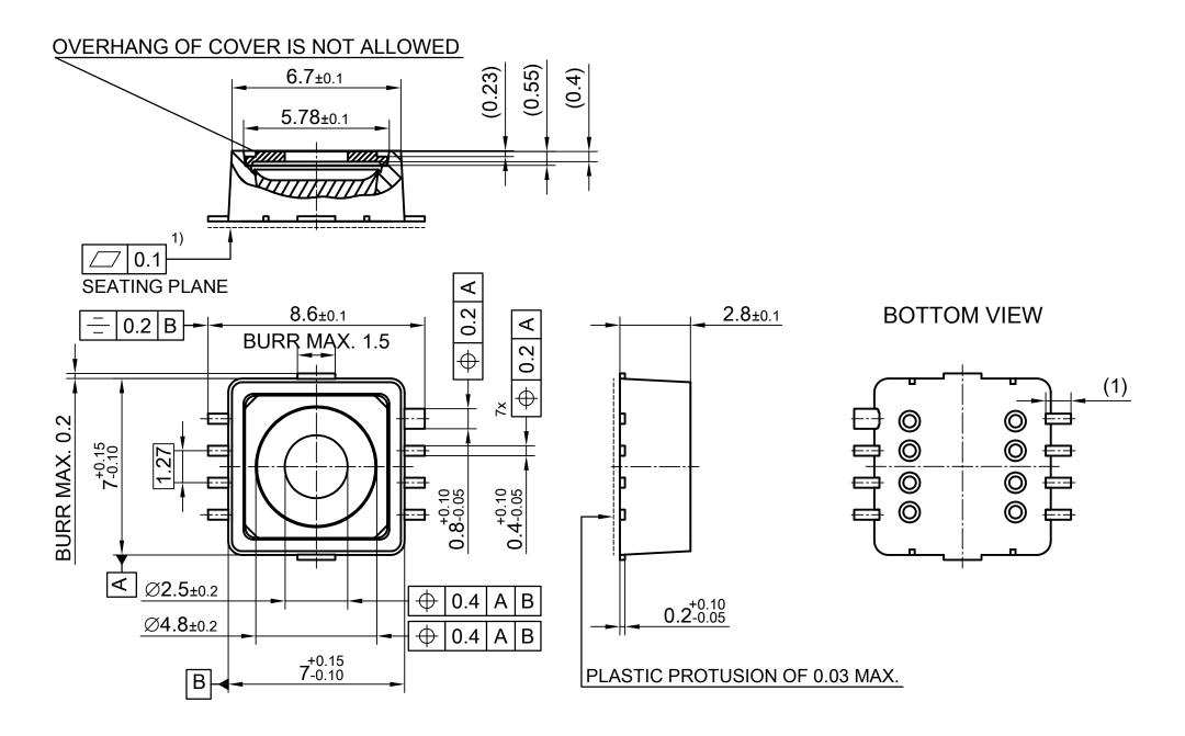
OUTER DIMENSION DOES NOT INCLUDE PROTUSION OR INTRUSION OF 0.2 MAX. PER SIDE 1) VALID FOR THE WHOLE SEATING PLANE INCLUDED TIEBAR AREA ALL DIMENSIONS ARE IN UNITS MM
