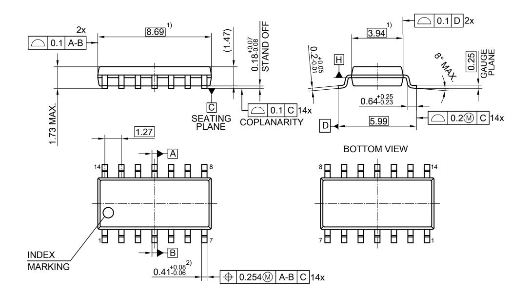
1) DOES NOT INCLUDE PLASTIC OR METAL PROTRUSION OF 0.25 MAX. PER SIDE 2) DOES NOT INCLUDE DAMBAR PROTRUSION OF 0.1 MAX. PER SIDE ALL DIMENSIONS ARE IN UNITS MM THE DRAWING IS IN COMPLIANCE WITH ISO 128 & PROJECTION METHOD 1 [
