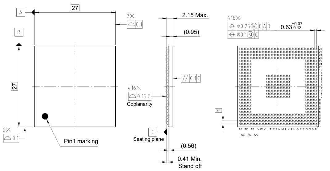
All dimensions are in units mm The drawing is in compliance with ISO 128-30, Projection Method 1 [ $\bigcirc \oplus$ ] Drawing according to ISO 8015, general tolerances ISO 2768-mK
