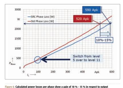
current with slew rate control (blue) over a standard driver (red) ( $V_{DC}$  = 600 V, -8 V <  $V_{GE}$  < 15 V,
