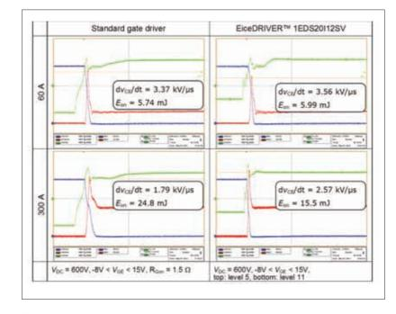
Figure 4: Large advantage of more than 40% with 1EDS0I12SV regarding turn-on energy compared to standard gate driver in a gate driver design example showing the collector-emitter voltage (blue), the collector current (red), and the gate-emitter voltage (green)
