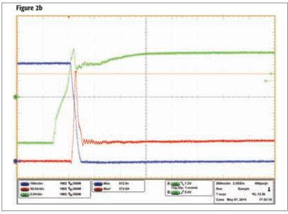
Figure 2: Commutation of low currents at 10 % of nominal current level (a:  $R_{Gon} = 0\Omega$ , b: RGon = 1.5 $\Omega$ ;  $V_{Dc} = 600V$ ;  $I_c = 60A$ ; -15V <  $V_{Gc} < 15V$ ) with collector-emitter voltage (blue), collector current (red) and gate-emitter voltage (green) with a standard gate driver
