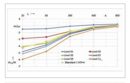
Figure 5: Example of  $dv\alpha/dt$  range (bottom) and turn-on energy  $E_m$  of 1EDS-SRC gate current control IC for speed level 1, 3, 5, 7, 9 and 11 compare to standard driver at IGBT junction temperature of 25°C
