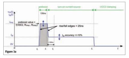
IGBT when it is operating at low collector current levels and it can also quickly turnon at high collector current levels. This is made possible by a user controlled current source providing 11 different levels. These levels can be selected by the system control pulse-by-pulse in real-time.
