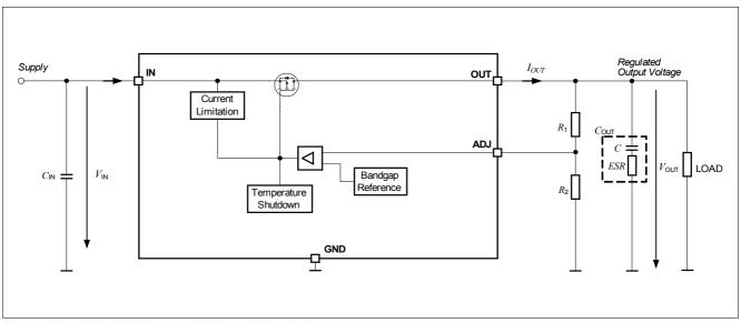
Figure 3 Block Diagram Voltage Regulation
