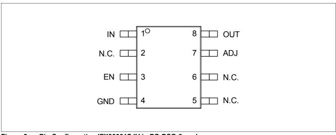
Figure 2 Pin Configuration IFX30081SJV in PG-DSO-8 package
