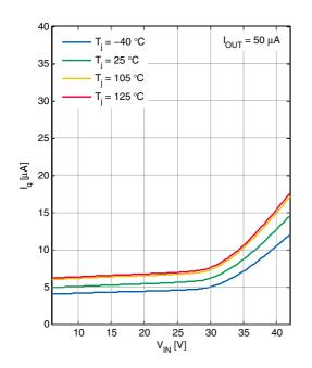
Current Consumption in OFF mode  $I_{\rm q,OFF}$  versus Input Voltage  $V_{\rm IN}$
