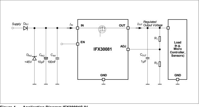
Figure 4 Application Diagram IFX30081SJV
