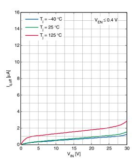
Current Consumption  $I_{\rm q}$  versus Input Voltage  $V_{\rm IN}$
