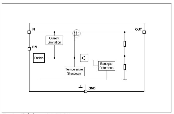
Figure 1 Block Diagram IFX30081LDV33
