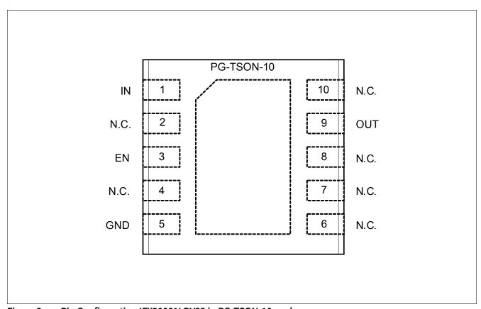
Figure 2 Pin Configuration IFX30081LDV33 in PG-TSON-10 package
