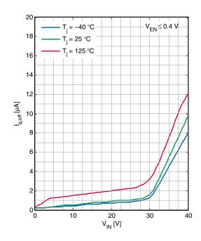
Current Consumption  $I_q$  versus Input Voltage  $V_{IN}$
