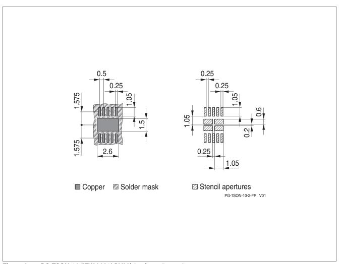
Figure 6 PG-TSON-10 (IFX30081LDV33) Package Footprint
