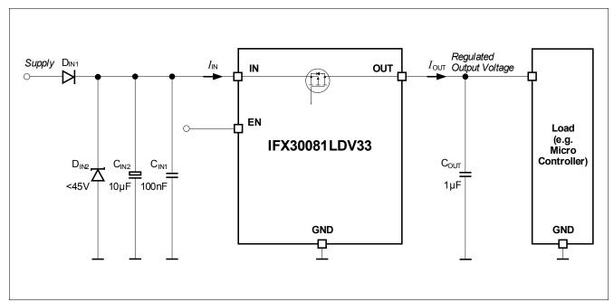
Figure 4 Application Diagram IFX30081LDV33
