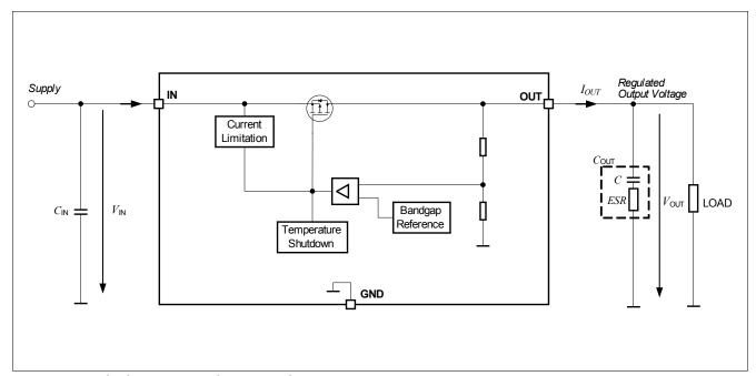
Figure 3 Block Diagram Voltage Regulation
