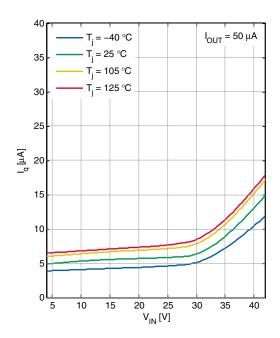
Current Consumption in OFF mode  $I_{\rm q,OFF}$  versus Input Voltage  $V_{\rm IN}$
