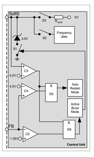
Figure 13 Adjustable Blanking Window
