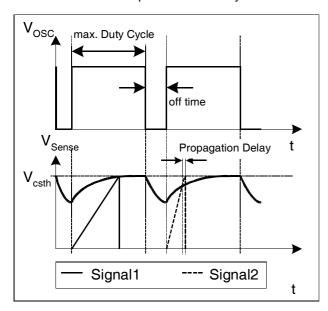
Figure 12 Dynamic Voltage Threshold V<sub>csth</sub>
