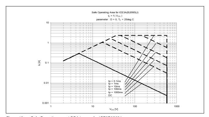
Figure 19 Safe Operating area ( SOA ) curve for ICE3B0565J
