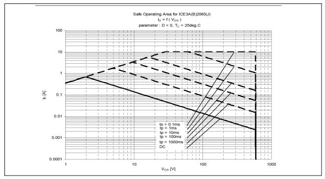
Figure 21 Safe Operating area ( SOA ) curve for ICE3B2065J
