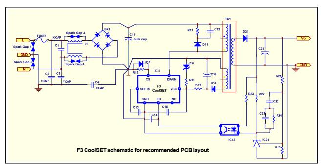
Figure 28 Schematic for recommended PCB layout
