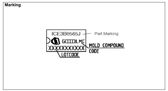
Figure 25 Marking for ICE3B0565J
