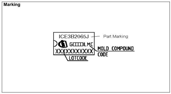
Figure 27 Marking for ICE3B2065J
