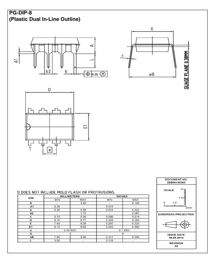
Figure 23 PG-DIP-8 ( Pb-free lead plating Platic Dual-in-Line Outline )
