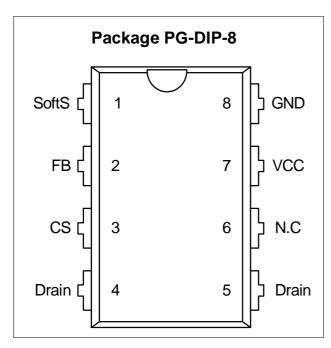
Figure 1 Pin Configuration PG-DIP-8(top view)
