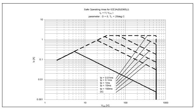
Figure 18 Safe Operating area (SOA) curve for ICE3B0365J
