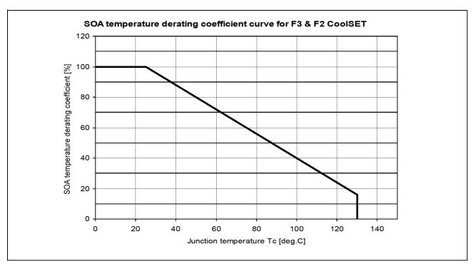
Figure 22 SOA temperature derating coefficient curve
