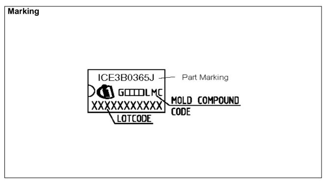
Figure 24 Marking for ICE3B0365J
