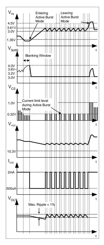
Figure 15 Signals in Active Burst Mode
