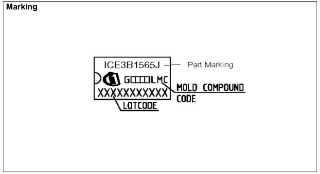
Figure 26 Marking for ICE3B1565J
