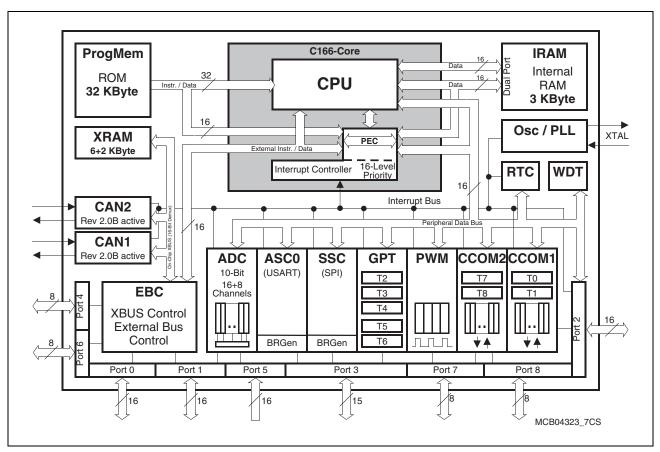
Figure 3 Block Diagram
