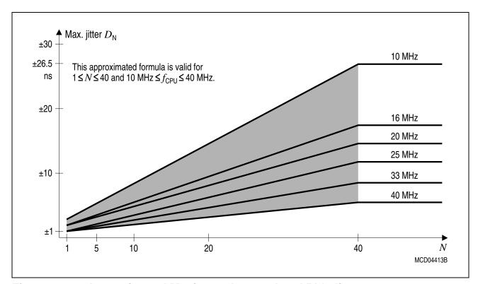
Figure 12 Approximated Maximum Accumulated PLL Jitter
