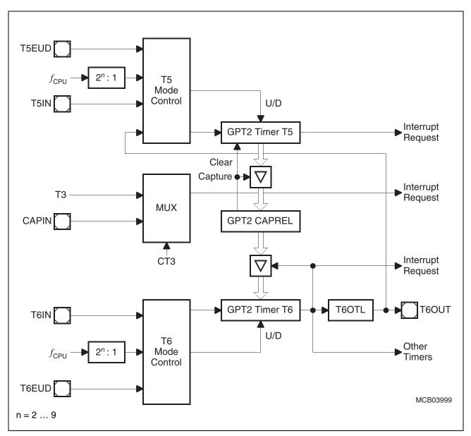
Figure 7 Block Diagram of GPT2
