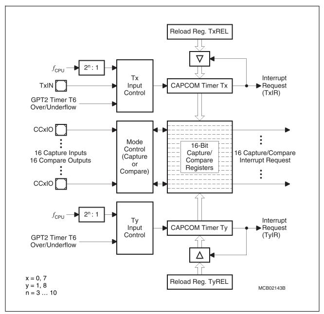
Figure 5 CAPCOM Unit Block Diagram
