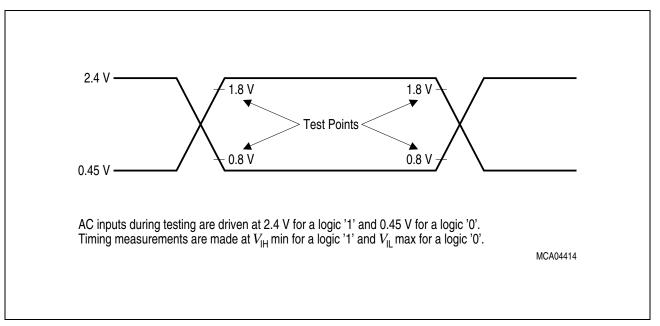
Figure 14 Input Output Waveforms
