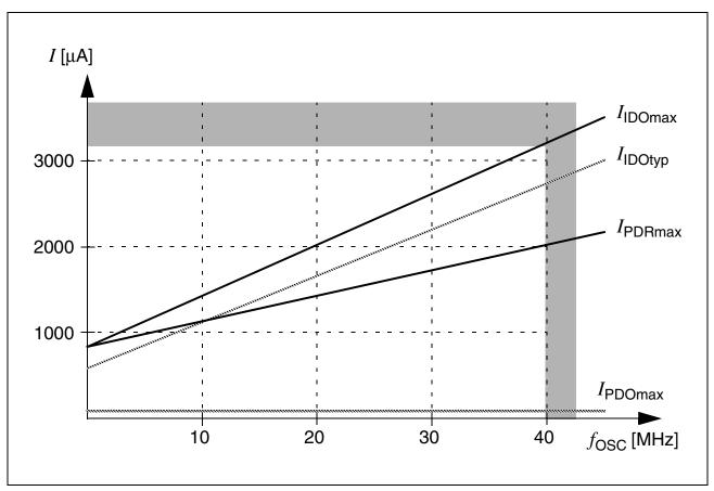
Figure 9 Idle and Power Down Supply Current as a Function of Oscillator Frequency
