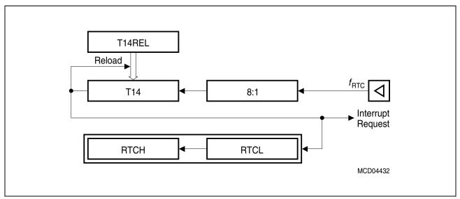
Figure 8 RTC Block Diagram
