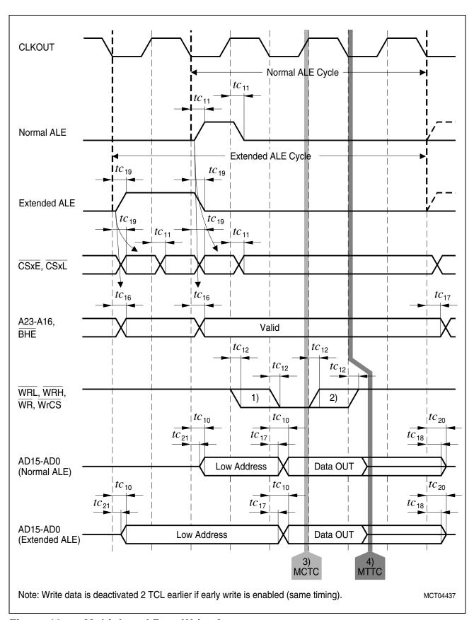
Figure 19 Multiplexed Bus, Write Access
