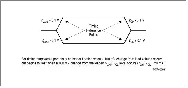
Figure 15 Float Waveforms
