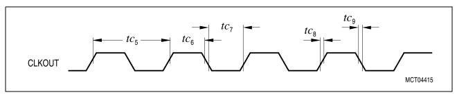
Figure 16 CLKOUT Signal Timing
