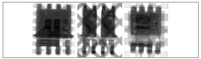
Figure 17 X-ray photographs of properly a soldered TDSON-8 (left), a TDSON-8 with dual pad (center), and a TSDSON-8 (right).
