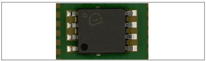
Figure 15 Photograph of a TDSON-8 with LTI solder joints on a test board. The different appearance of the gate and source leads on the left side compared to the leads fused with the pad on the right side is visible.
