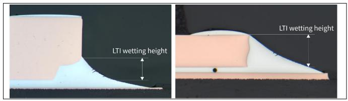
Figure 7 Cross section of a soldered trapezium groove LTI on the HSOF-8 (left) and of a soldered fully plated LTI on the TDSON-8 (right).
