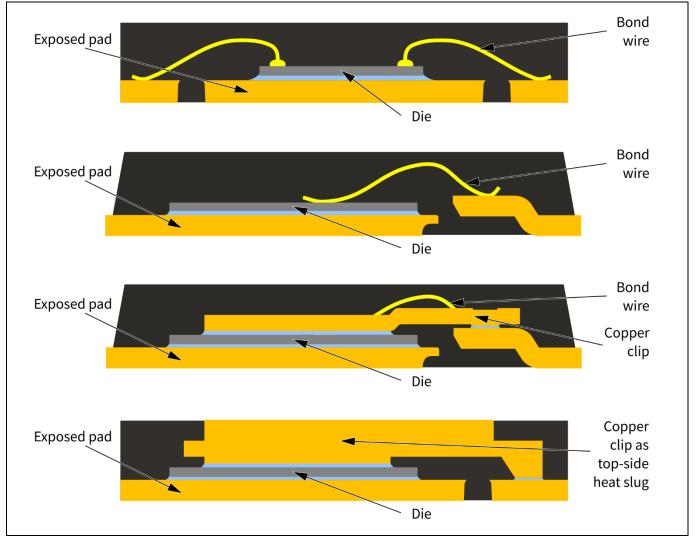
Figure 4 Schematics showing the inner setups (from top to bottom) of a configuration with twoside wire bonds, with one side wire bond, with a combination of copper clip and wire bond (also with copper clip only possible), and with a copper clip that is extended to a heat slug for enabling top-side cooling.
