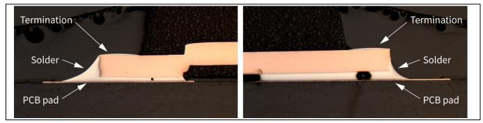
Figure 16 Cross section of a TDSON-8 assembled on board. The natural tilt of the package is visible causing the different appearance of the solder joint fillet on leads that are fused with the pad (right) compared to the single ones (left). However, the LTI tips are wetting properly on both sides.
