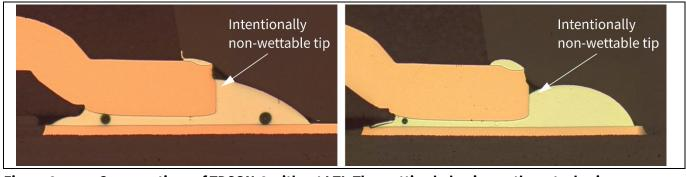
Figure 6 Cross sections of TDSON-8 without LTI. The wetting behavior on the cut edge is inconsistent.
