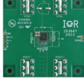
Figure 1: Reference Board SupIRBuck 25 A solution
