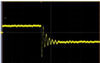
Figure 3a: Transient waveform before optimization
