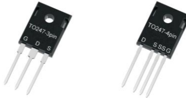
Fig. 1 TO-247 package and TO-247 4pin package with Kelvin source connection (source sense (SS))
