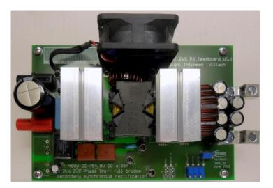
Figure 3.3: Infineon's 2kW ZVS full bridge phase-shifted DC-DC converter
