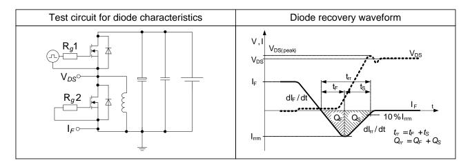
Figure 2.3: Infineon's hard commutation test circuit and diode recovery waveform
