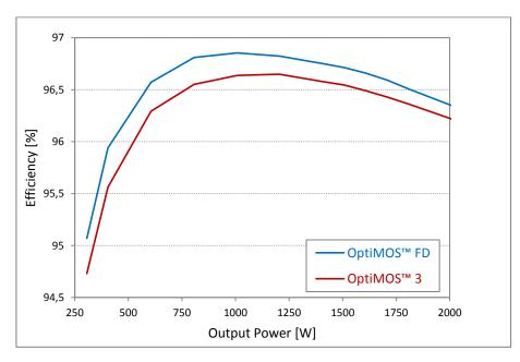
Figure 3.4: Efficiency comparison between OptiMOS<sup>™</sup> FD and OptiMOS<sup>™</sup> 3
