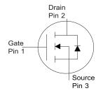
Figure 2.1: Symbol of a Power MOSFET
