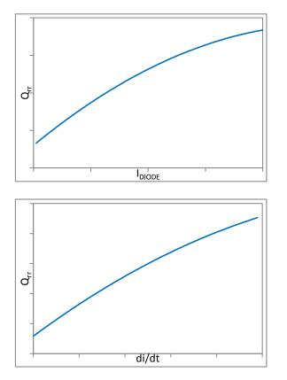
With di/dt fixed, the higher the body diode conduction current, the higher the stored  $Q_{rr}$  in the device.
