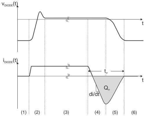
Figure 2.2: Operation of a diode [1]
