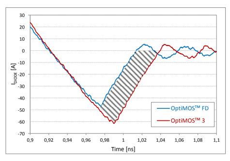
Figure 3.1: Experimental waveforms of reverse recovery current
