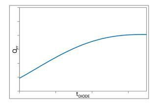
Reverse recovery charge accumulates over time. At a fixed diode conduction current and di/dt,  $Q_{rr}$ accumulates in the MOSFET during body diode conduction. The longer the body diode conduction time, the more charge is accumulated until it saturates.
