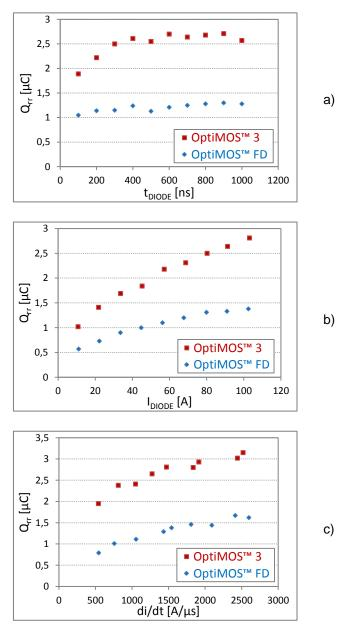
Figure 3.2: Q<sub>rr</sub> Measurements (a) Q<sub>rr</sub> vs t<sub>DIODE</sub> @I<sub>DIODE</sub>=100A and di/dt=1000A/µs; (b) Q<sub>rr</sub> vs I<sub>DIODE</sub> @di/dt=1500A/µs and t<sub>DIODE</sub>=300ns; (c) Q<sub>rr</sub> vs di/dt @I<sub>DIODE</sub>=100A and t<sub>DIODE</sub>=300ns.
