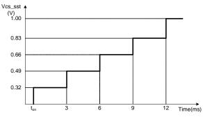
Figure 4 Maximum current sense voltage during softstart
