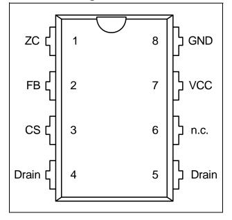
Figure 1 Pin Configuration PG-DIP-8 (top view) Note: Pin 4 and 5 are shorted
