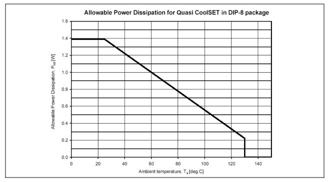
Figure 10 Power dissipation;  $P_{tot}=f(T_a)$
