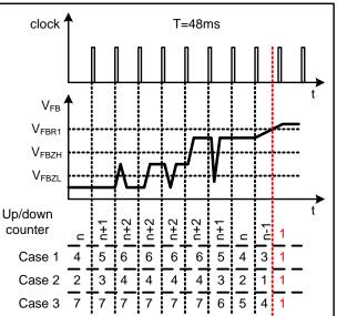
Figure 5 Up/down counter operation
