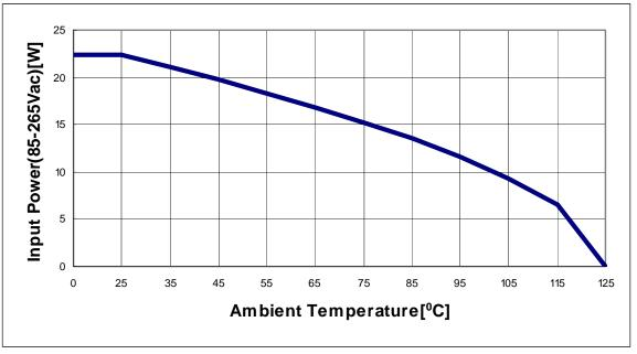
Figure 12 Input Power curve Vin= $85 \sim 265$  Vac; Pin= $f(T_a)$
