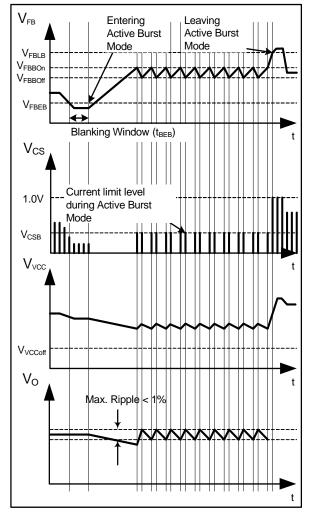
Figure 8 Signals in Active Burst Mode
