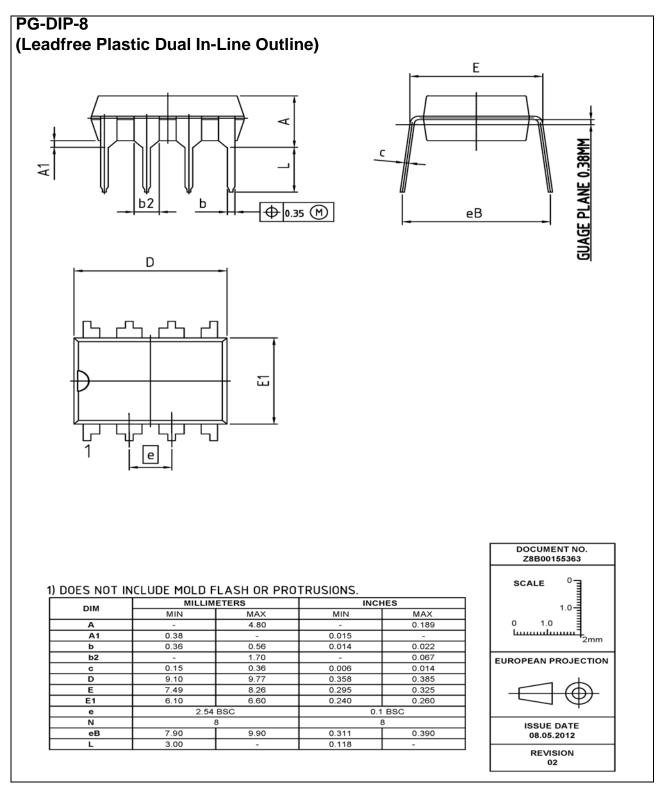
Figure 14 PG-DIP-8 (Pb-free lead plating Plastic Dual-in-Line Outline)
