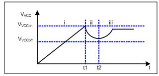
Figure 3 VCC voltage at start up
