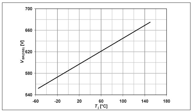
Figure 11 Drain-source breakdown voltage;  $V_{BR(DSS)}=f(T_j)$
