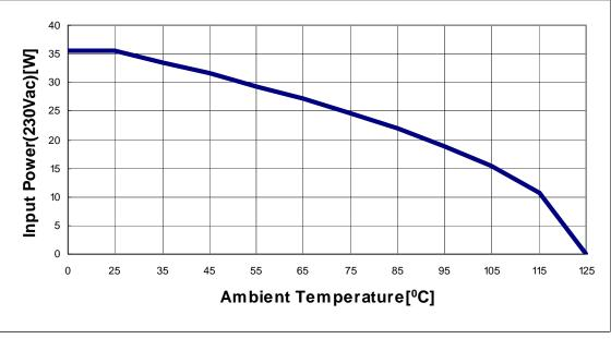
Figure 13 Input Power curve Vin=230Vac;Pin= $f(T_a)$
