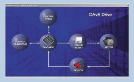
Graphical User Interface of DAVE Drive Infineon's DAVE and DAVE Drive are GUI based configuration tools and source code generators. DAVE Drive let's you select motor type, motor speed and torque.
