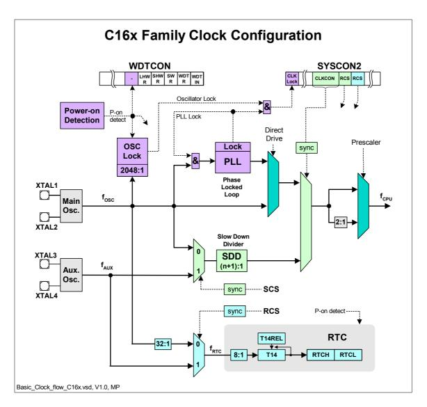
Note: The C161PI includes no auxiliary oscillator. Bits SCS and RCS are set to zero.
