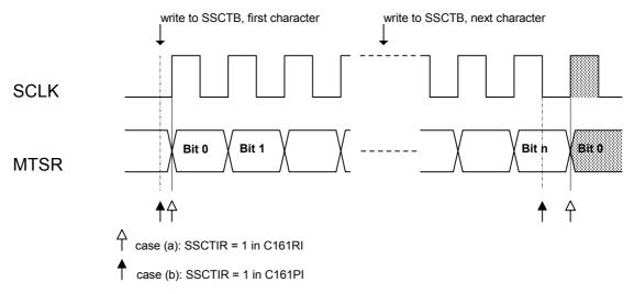
Typically, in interrupt driven systems, no problems are expected from the modified timing of flag SSCTIR. However, when flag SSCTIR is polled by software in combination with other flags which are set/cleared at the end or at the beginning of a transfer (e.g. SSCBSY), the modified timing may have an effect.
