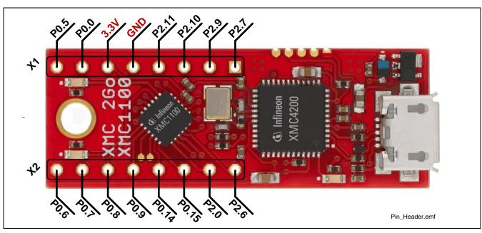
Figure 3 Pinning of pin header
