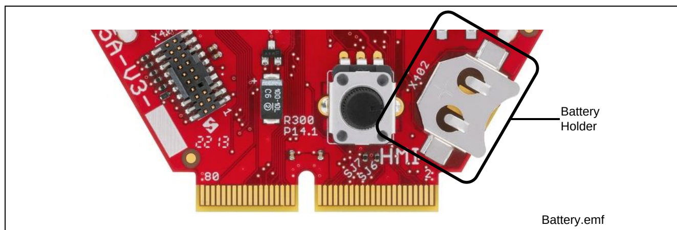
Figure 5 Battery (VBAT Supply)
