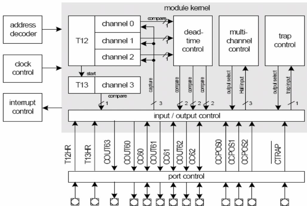
**Figure 5. CCU6 Functional Block Diagram**
