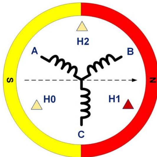
**Figure 2. Single pole pair BLDC motor with hall sensors**
