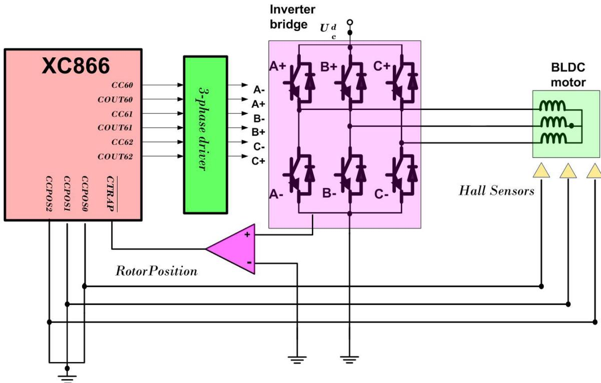
Figure 4. BLDC motor driver with hall sensors
