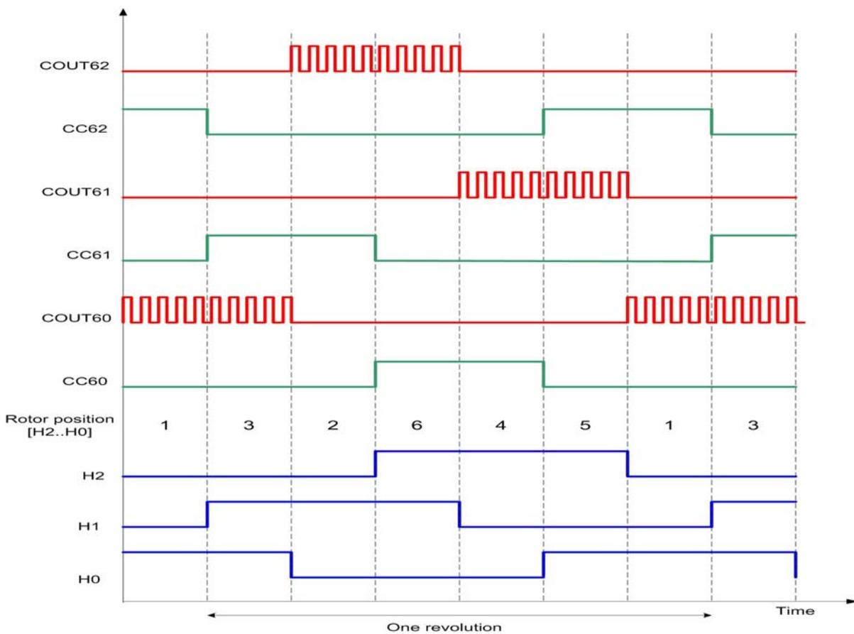
**Figure 6. CCU6 output signals and Hall pattern**
