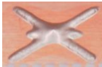
Dispense Patterns Visible solvent bleed out
