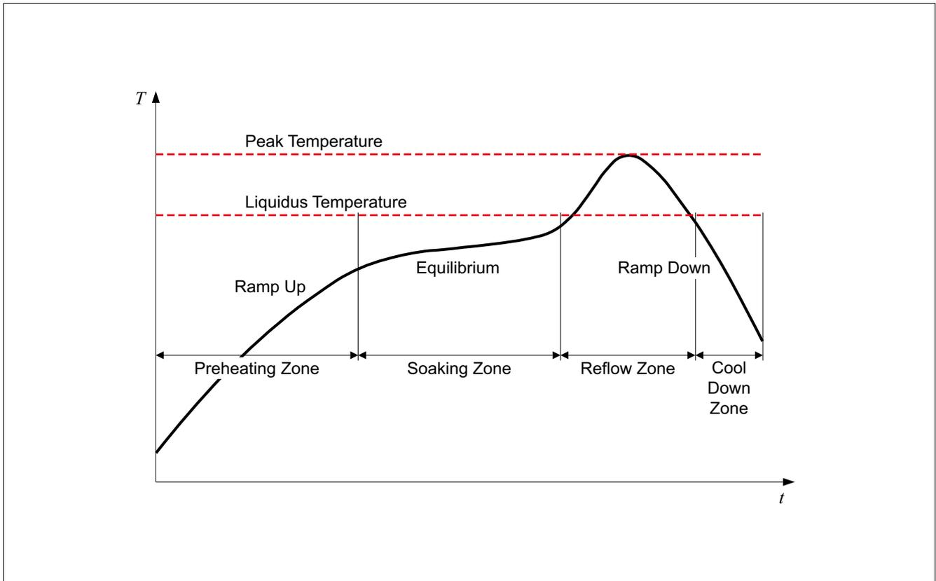
**Figure 5** General Forced Convection Reflow Solder Profile
