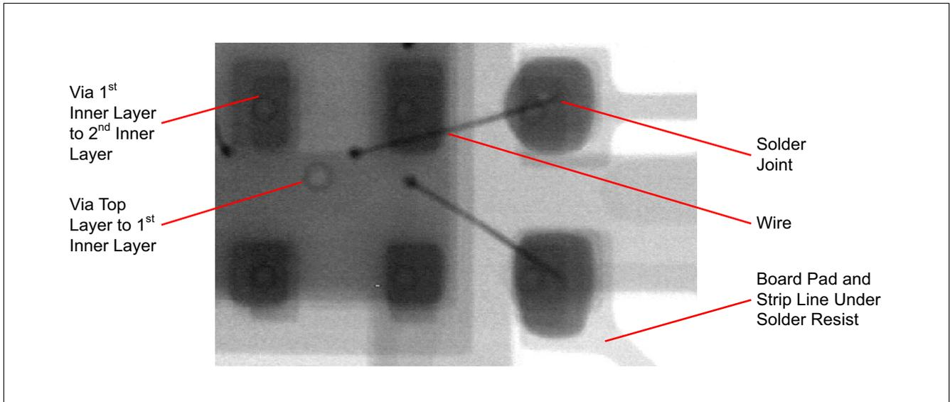
**Figure 7 Typical X-ray Image of a Soldered TSLP.**
