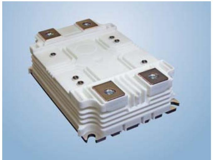
Figure 4: Defining a new industrial standard, the high-power platform „The Answer“ for several voltage classes from 1200V up to 6.5kV, among others with 400A for 4.5kV and 275A for 6.5kV, and a dimension of 100mm x 140mm x 40mm
