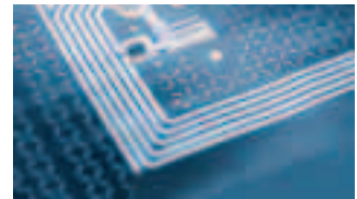
RFID tags with chip and aerial
