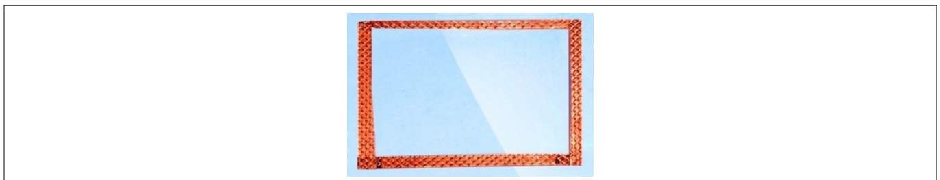
Figure 13 Proximity sensor prototype using copper tape as wire loop
