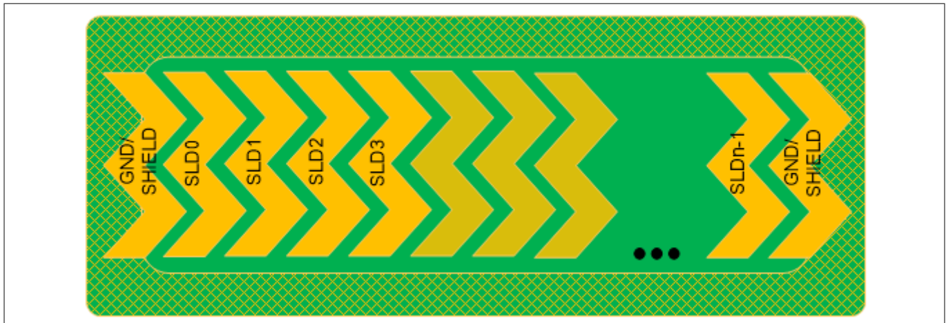
Figure 146 Linear slider pattern when first and last segments are connected to top hatch fill
