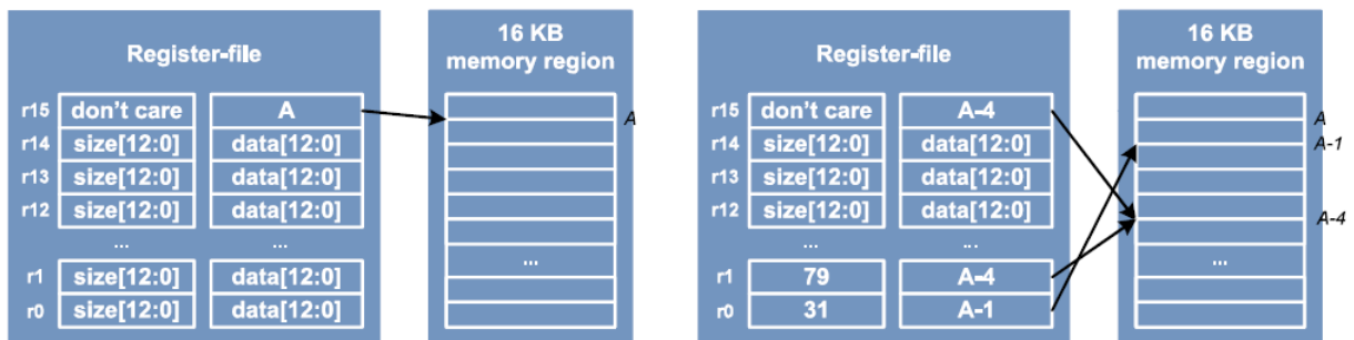
Figure 11-18. Left: Register File State before ALLOC_MEM Instructions; Right: Register File after ALLOC_MEM Instructions
