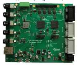
family, while supporting the latest communications interfaces, featuring a Gigabit Ethernet interface, multiple ISO 11898-1-compliant CAN FD channels, as well as LIN and Flexray channels. An additional eMMC interface for external flash interfacing enables local data storage, supporting software-over-theair update concepts. Realtek's RTL9047AA automotive Ethernet switch controller features five integrated
