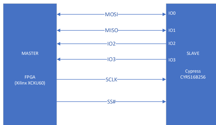
Figure 2. QSPI configuration connection with SPI Flash
