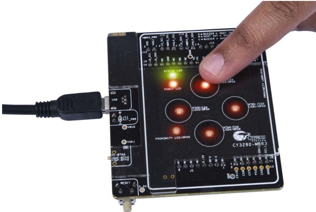
Figure 5-8. LEDs with 93 Percent Brightness on Button Touch
