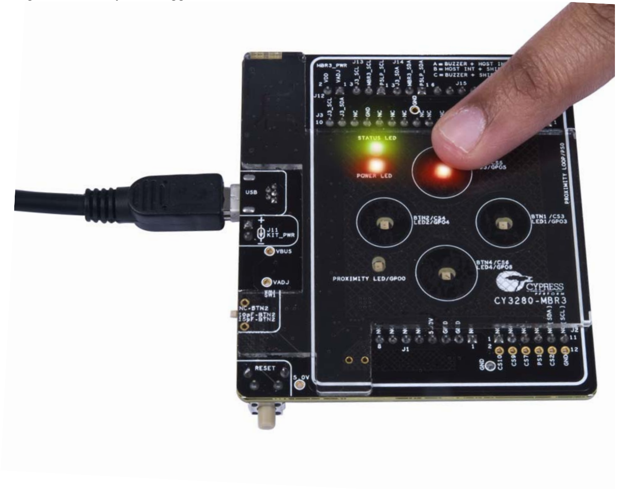
Figure 5-6. Verify LED Toggle Feature
