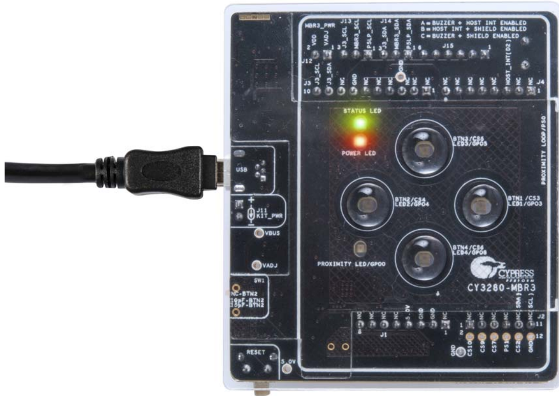
Figure 5-17. Verify Water Tolerance - Without Finger
